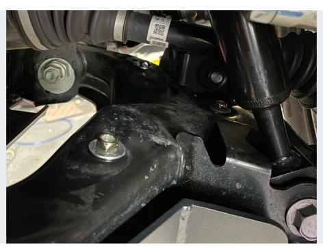
With the skid lined up to each of the (3) holes, insert a carriage bolt though the bottom of the skid up through the control arm, with a washer and nylock nut on top. Leave everything loose.
