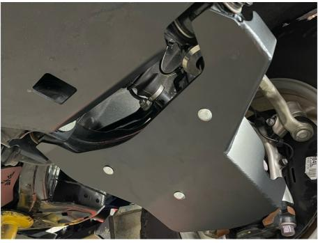
With all of your bolts started, use a wrench to tighten them all down into place. Repeat this same process on the other control arm to complete your install.
