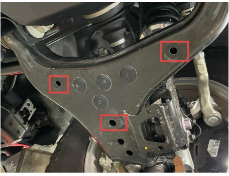
The (3) holes shown above will be used to mount the lower control arm skid to the lower control arm.
