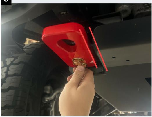
Next, using (2) of the supplied M12 bolts and washers, loosely install the Victory 4x4 Billet Recovery Point into the factory holes. Be sure to square up the part with the vehicle, and then tighten with a 19mm socket. Repeat on the other side of the vehicle.
