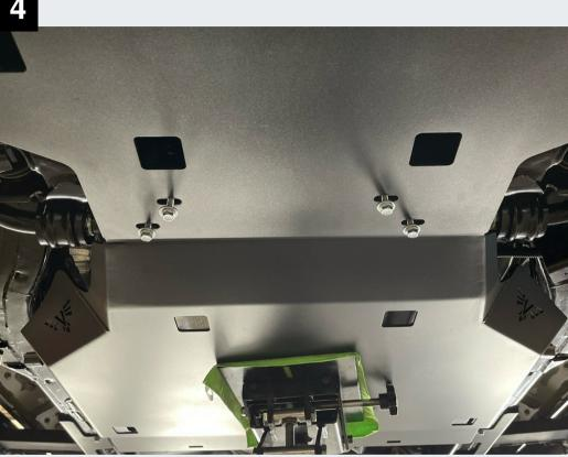
Begin by removing the plastic cover from the cross member. The points indicated in the image must all be pushed in to remove the cover.
