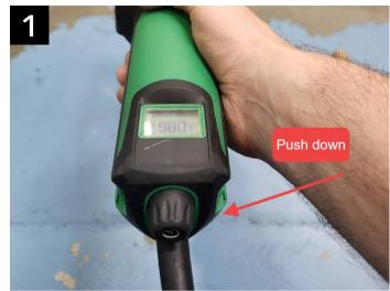
Ensure Leister is plugged in. Hold bottom button pressed Turn dial to desired temperature. in till you hear it turn on.
