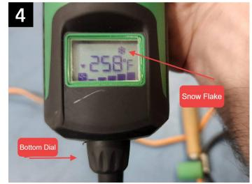
Check weld. To turn off Liester press and hold bottom dial until a snowflake appears on the display. Wait for cooldown.
