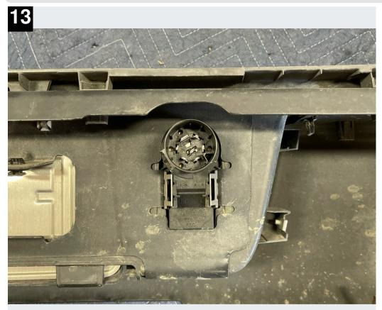
Push in on the metal tabs on either side of the trailer plug and push it through the bumper.
