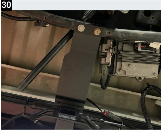
If not installing carriers, plastic plugs can be installed into the spindle sleeve. it If keeping the spare tire in the factory location, install the provided bracket is best to put a little bit of RTV around the rim to make a weatherproof seal on the sleeve in case carriers are installed later.
