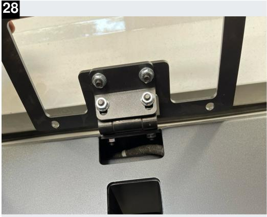
Bolt the small angled bracket onto the back of the license plate bracket and then, mount the side of the hinge with the bolt in it to the top of the angled bracket as well. The license plate bracket assembly can then be bolted onto the bumper with the 1/4" hardware. The nuts on the back can be installed through the cutout.
