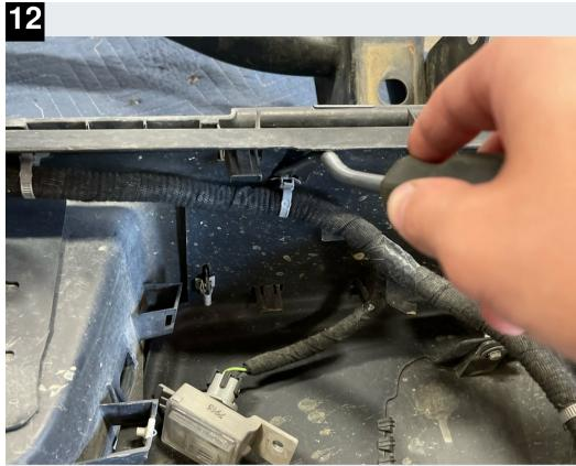
Remove the bolt holding each light to the bumper and remove both lights from Remove all clips and pull wiring harness out of the bumper. their retainers.
