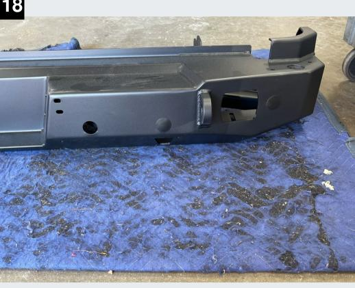
Bolt the light and bracket to the inside of the bumper using the 1/4" hardware. The end with the bolt should be on the bottom as shown.
