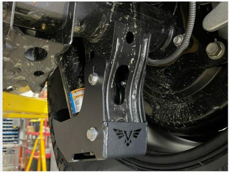
Once all (4) of your bolts are started into the nut tabs and the height is adjusted, use a 1/2" wrench and tighten them all down to finish your install.
