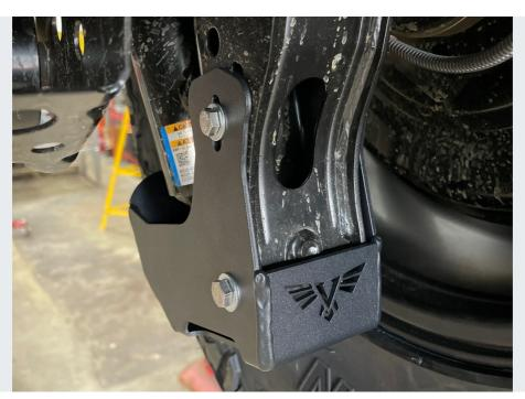
Take the provided hardware and insert it through the skid into the holes stated in the previous step on each side of the skid. There is a slot in the skid to adjust height.
