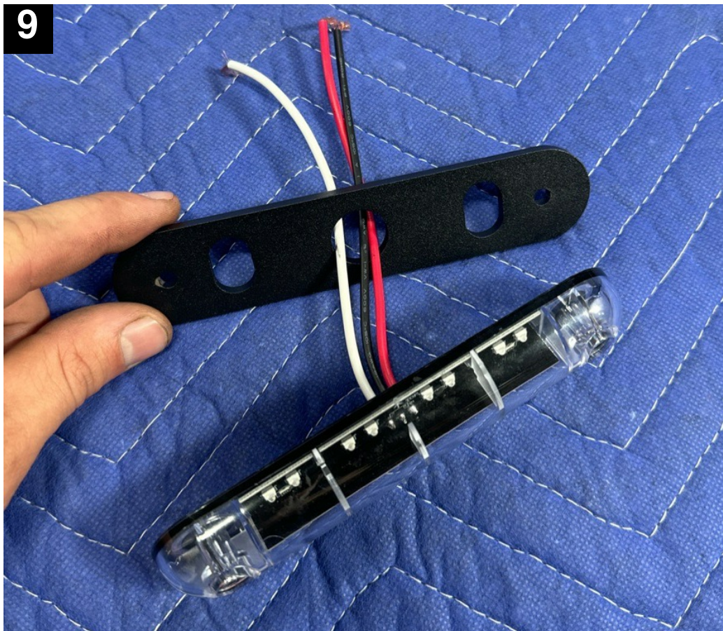
Pass the wires through the center hole in the light spacer.
