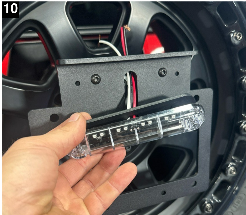
Then pass the wires through the wire hole/cutout on the mounting bracket.
