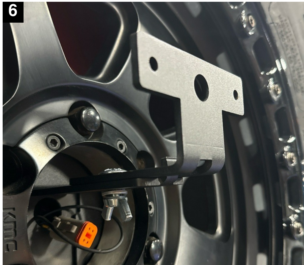
Next install the outer bracket half as shown, secure it using the 3/8" carriage bolt, split washer and wing nut.
