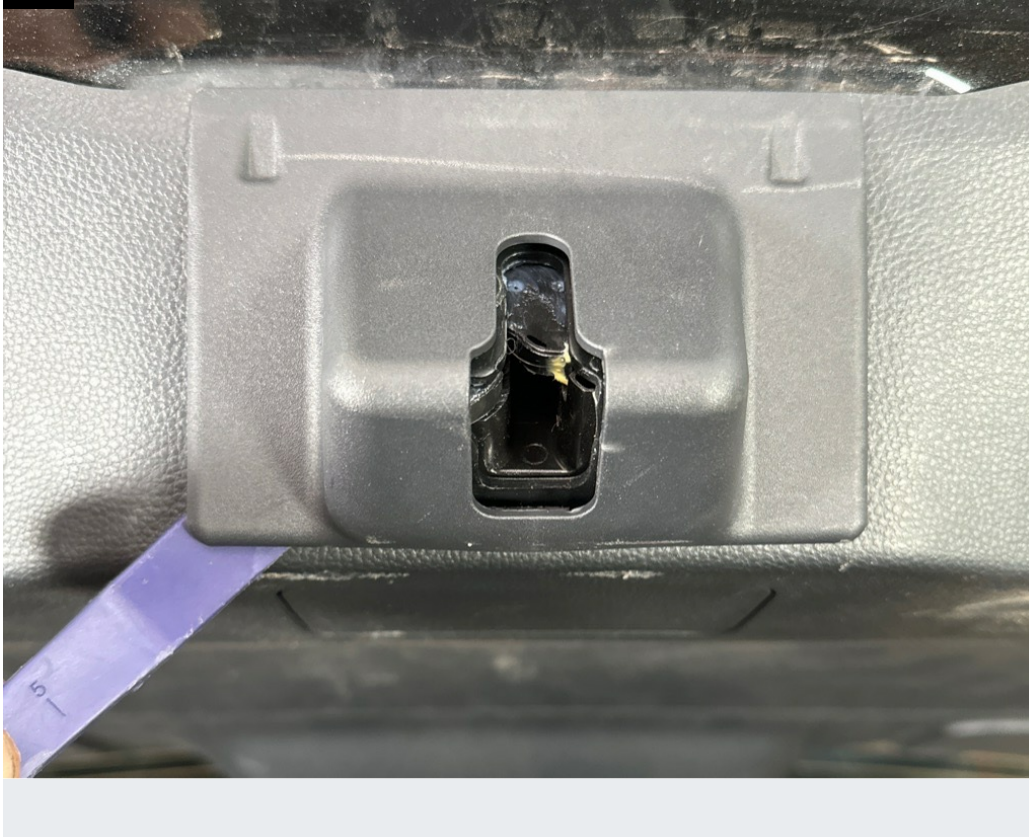
Pry from the bottom and pivot out to release the center latch cover.
