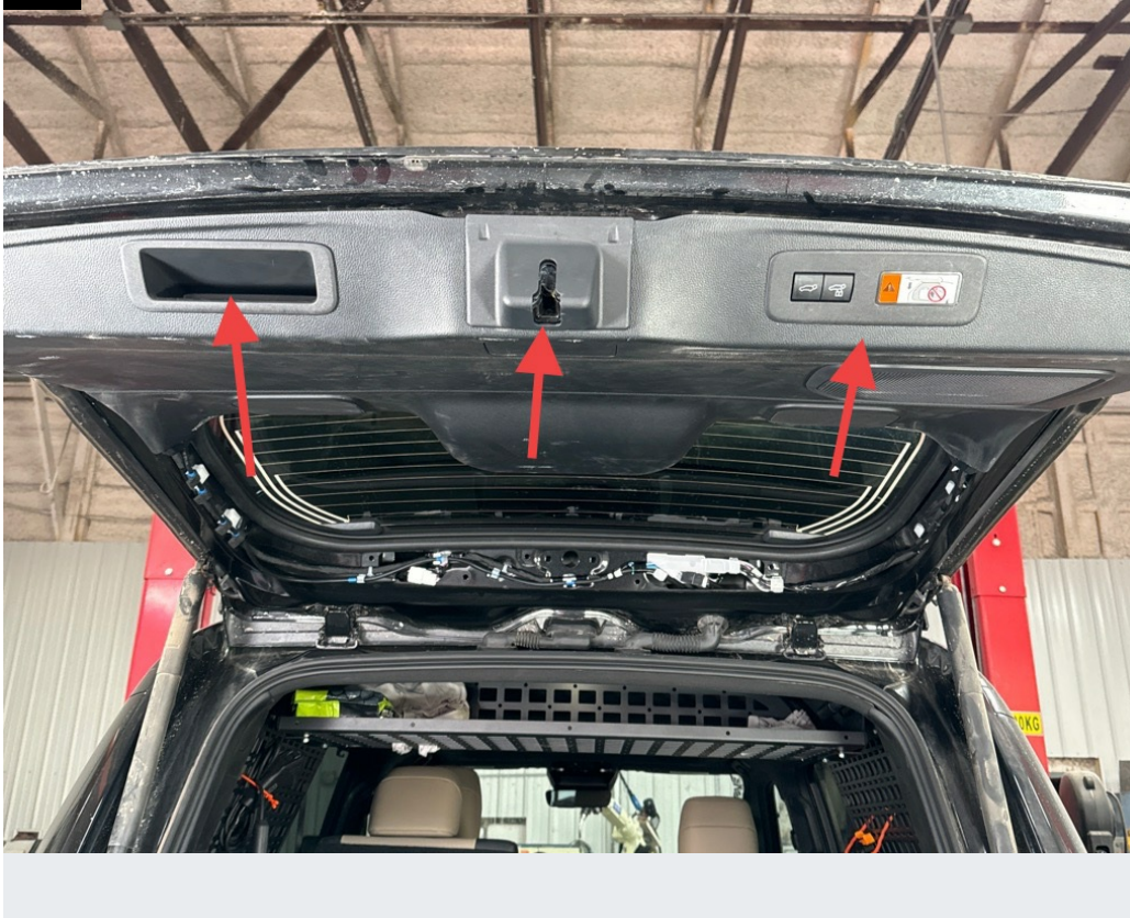
At the base of the hatch you need to remove the 3 plastic panels shown here.
