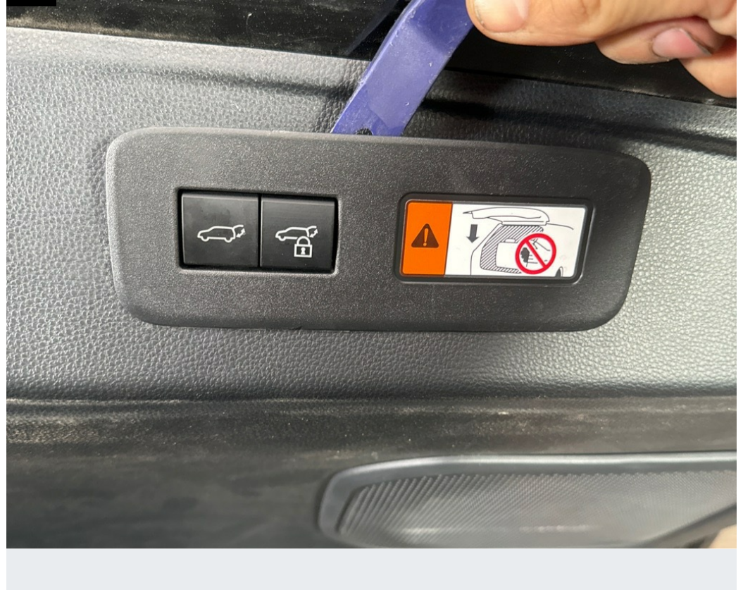
Pry from the top of the switch plate and pivot out to release the panel.
