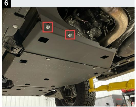
Set the skid up into place with the provided spacers between the top of the skid and the frame. If installing with our Transmission Skid, the TCase Skid should sit between the Transmission Skid and the spacers. Once in position, the skid can be held loosely in place using the 1/2" carriage bolts with the provided square washer, flat washer and nylock nut on the top of the frame, in that order.
