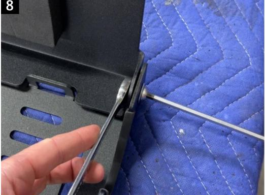
To mount the door, insert a 5/16" button head through the 1/4" USS washer, mounting plate, nylon washer and door in that order with on of the 5/16"-18 nylon insert locknuts on the other end as shown in the image. Repeat this for the other four mounting holes. It can be helpful to use something thin and flat such as flat head screw driver to help position the nylon washers.
