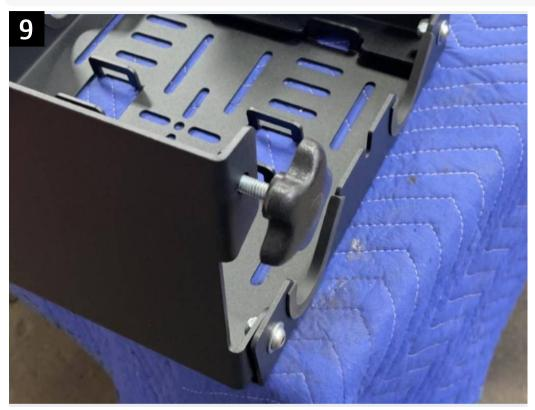
Thread the knobs part way into the nuts in the doors. The knobs are used to secure the doors to the base plate in the closed and ensure they do not open unintentionally.
