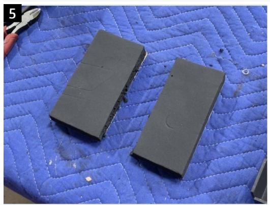
Cut the foam as desired for your specific application. This will help to hold the tools in place without any movement. Simply cutting the square in half is a safe bet for many applications.
