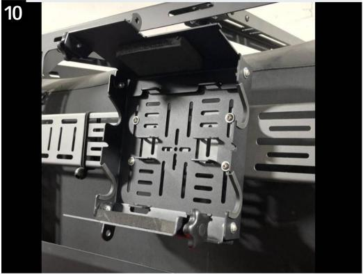
The remaining bolts are provided for mounting. Depending on what you are mounting to, different slots may need to be used and different hardware may need to be sourced. The bent tabs on the mounting face can be used for straps, bungee cords, or other similar thing as needed.
