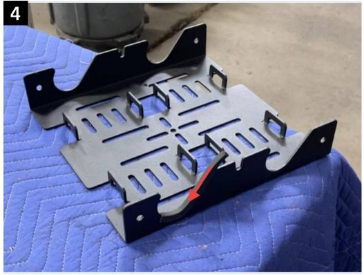
Slide the edge trim onto each of the four cutouts in the mounting plate. It is easiest to start on the longer edge and push the trim around the radius following the arrow shown in the image.
