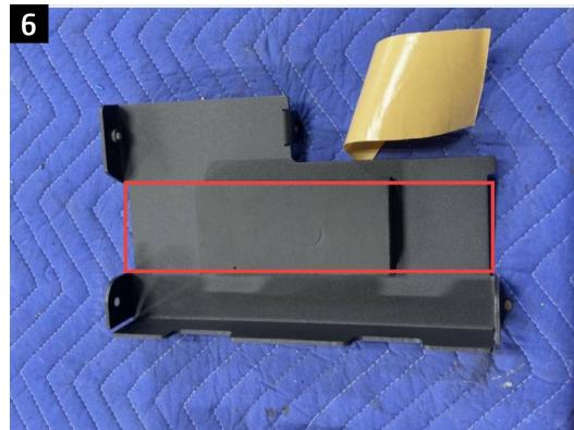
Peel the backer off the foam and stick it to the inside surface of the door in the desired position. This will most likely be in the position shown in the image. Keep in mind that the tool will sit in the red boxed area.
