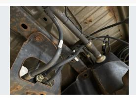
NOTE: Use caution while lowering and maneuvering not to impose undue tension or other forces onto fuel lines, filler neck, or EVAP lines.
