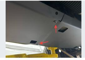
Bolt the two skid halves together using (2) 3/8"-16 x 3/4" black button head screws and 3/8"-16 flange lock nuts. Tighten these fully.
