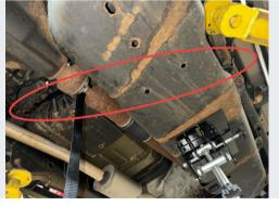
Use a second ratchet strap and repeat the same process to suspend the rear of the tank.
