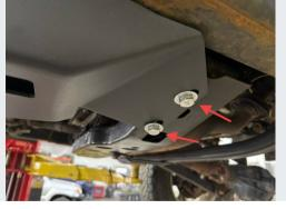
Use the remaining (2) M12 screws to attach the front of the skid to the transmission crossmember.
