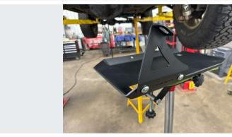
Loosely pre-install the bracket #1 onto the rear, outside corner of the rear skid half using (2) 1/2" x 1" button head bolts and 1/2" flange nuts as shown.
