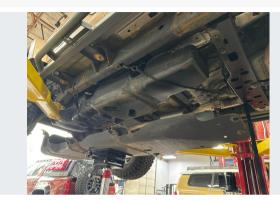
With the tank fully supported, lower the jack and factory tank skid completely out of the way and remove.
