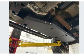
Verify that the entire assembly is situated properly and begin tightening all of the remaining loose hardware.
