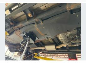
With the last two fasteners retaining the factory tank skid, support the entire assembly with a jack positioned near the middle.
