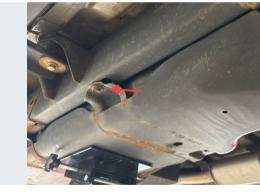
Remove the final fasteners: (1) near the front of the skid on the outside, into the frame rail.
