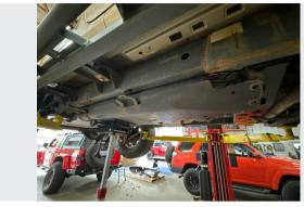
Carefully lower skid and tank assembly just enough to allow it be moved freely. Only a couple of inches is necessary.
