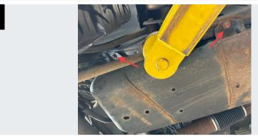
Remove the middle and rear fasteners on the outside of the tank skid.
