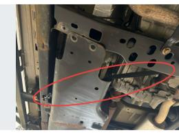
Slip a ratchet strap between the fuel tank and the factory tank skid, connecting to the frame and a point opposite so that the strap may be tightened to suspend the tank.
