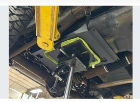
Using the jack, lift the rear portion of the JCR tank skid into place with the jogged flange oriented to the front of the vehicle. Support the tank with the skid and remove the ratchet strap.
