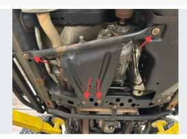
Remove (4) bolts retaining the transfer case skid using an 18mm socket
