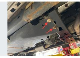
Remove front (2) bolts retaining factory tank skid to transmission crossmember.
