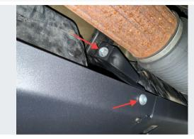
Attack bracket #3 to the middle of the front skid half on the inside mounting hole with a 1/2" x 1" button head screw and flange nut, and to the factory skid mounting point on the crossmember above with another M12 screw and flat washer.
