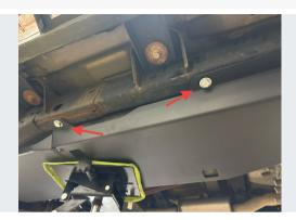
Use (2) M12 screws and flat washers to loosely attach the outside of the skid to the factory locations on the frame.
