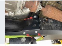
Attach bracket #4 to the skid using (2) 1/2" x 1" button head screws and nuts, and to the factory mount on the crossmember advice with another M12 screw and flat washer.
