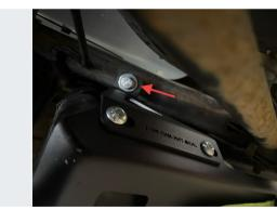
Attach the bracket to the frame in the factory rear outside mounting location using an M12 x 1.5mm x 30mm and flat washer. Start but do not tighten.
