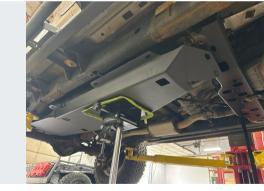
Raise the front skid half into place, supporting the tank, and remove the front ratchet strap.
