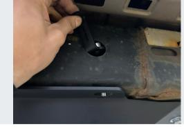
Insert the included nut-tab into the hole in the frame above the hole that was just drilled.
