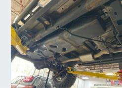
Reposition and adjust the straps supporting the tank. With the assistance if the jack tighten them up slightly to help draw the tank back into the original position.
