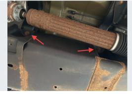
Remove the front and middle fasteners on the inside of the factory tank skid.
