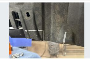
Refund the cut further, as shown. Ensure that the "flap" that will remain hanging down overlaps the spot in the back of the viper wing.
