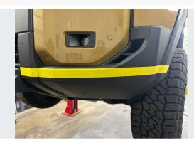
To prepare for marking out the cut, lay out a piece of wide painters tape along the edge of the lower filler panel where the "vertical" face meets the "horizontal" face as shown.
