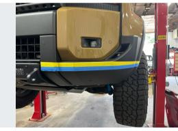
Use a second color tape, or a lockable laser level and marker, to connect the plotted points in the fascia and connect them to produce a cut line.
