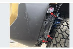
Remove (2) remaining clips and (1) screw beneath the flare.
