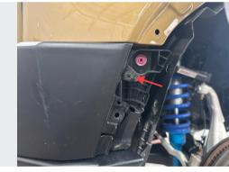
Reinstall the screw to retain the corner of the fascia on each side.
