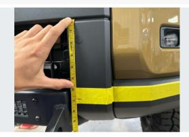
Using a flexible tape measure, measuring from the crease at the top of the lower grill surround as shown in the image, make a mark on the tape at 6-3/4" at the edge closest to the Blitz bumper.
