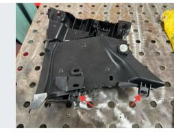
Begin splitting the inner and outer shell of the radar bracket by releasing the two clips at the bottom of the assembly as shown.
