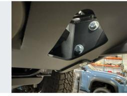
Tighten the two initial mounting bolts once the outer bolts are tightened.
