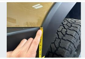
Posting the tape at the intersection of the upper and lower panels where they meet the flare, as shown. Let the tape fall vertically and confirm it to the contour of the flare.
