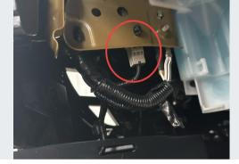
Reconnect the main harness on each side. Tidy and tie up the loose wiring harness before registering the inner fender.
