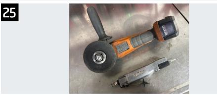
To make the cut you may use a small reciprocating saw or a cut-off tool with an abrasive disc. Always wear safety glasses and protective equipment when performing these operations Before cutting the fascia, ensure that all wires and other sensitive parts are clear from behind the marked area. Alternatively, the fascia may be removed entirely to perform the cut off of the vehicle entirely.
