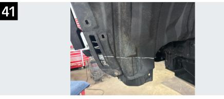
Using the Viper wing as a guide, mark the inner fender for the initial trim.
