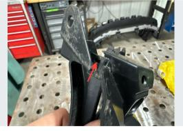
Use a small screwdriver to releases a third clip found at the lower rearward corner of the assembly.
