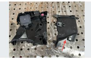
Retain main portion the bracket to reinstall after fascia is trimmed. Inner section may be discarded.
