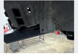
Using the slot as a guide, drill first and 1/8" hole and then a 3/8" hole in the inner fender to accommodate the included clip nut.
