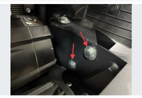
Bolt the wing to the Blitz bumper outside upright using (2)  $1/2 \times 1^{"}$  hex head screws, flat washers, and  $1/2^{"}$  flange lock nuts. Snug but do not fully tighten.
