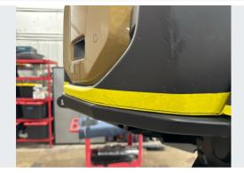
Use the wing as a guide to mark the fascia to create an even cut with approximately 1/8"- 3/16" gap.
