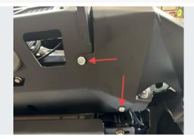
Bolt the bottom of the Viper wing to the Blitz bumper using (2) 1/2" x 1" button head screws and more flange lock nuts. Snugs these up and verify the wing is fitting correctly before fully tightening.
