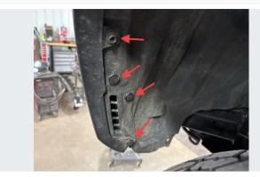
Remove (1) screw and (3) clips retaining inner fender to bumper fascia and lower portion of fender flare.
