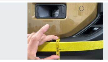
Make a third 2-1/8" mark where the panel starts to sweep upward, using the same method as the prior two.
