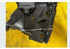
Mark radar mounting bracket as shown. Use reference features to create a cut line across the bottom of the bracket.
