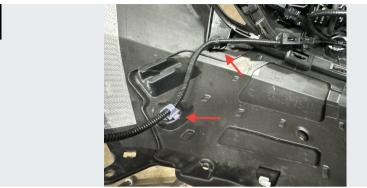
Disconnect the wire harness retainers from the inside of the fascia as indicated above.
