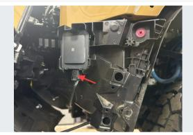
Unsnap the fascia from each side, and disconnect the corner radar.
