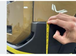
Holding the end of the tape flush with the top horizontal face of the lower fascia panel, and flat in the "bevel" let the tape fall vertically and conform it to the contour of the panel.
