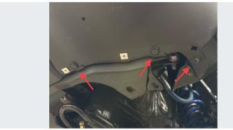
Remove (2) clips and (1) screw retaining the bottom of each of the lower fascia corner panels.
