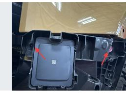
Remove the screw And rehearse the retainers holding the radar/fascia mounting bracket from the steel substructure.
