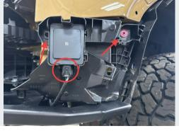
Reinstall the radar and bracket, and reconnect the harness.
