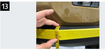
Repeat that measurement and mark at the "corner" of the lower filler panel as shown.
