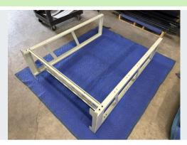
Install opposite side rack upright into existing shelf/upright assembly, install bolts and nuts, leaving them slightly snug.
