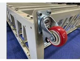
Install all 4 swivel casters onto mounting pads located on the bottoms of the rack uprights.
