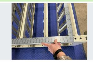
Use a framing square to check that the rack is square at each corner. Once this is verified. Beginning tightening all of the fasteners on the front of the rack.
