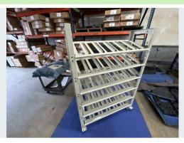
With the rack standing vertical, verify that it is still square and tighten the remaining fasteners on the back of the rack.
