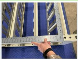
Use a framing square to check that the rack is square at each corner. Once this is verified. Beginning tightening all of the fasteners on the front of the rack.
