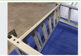
Ensure that the front shelf flange is aligned with the front of the rack. The angle of the shelf should be parallel to the angle of the cutouts in the rack upright. Internal forced flanges should face up.
