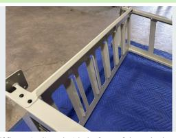
Ensure that the front shelf flange is aligned with the front of the rack. The angle of the shelf should be parallel to the angle of the cutouts in the rack upright. Internal forced flanges should face up.
