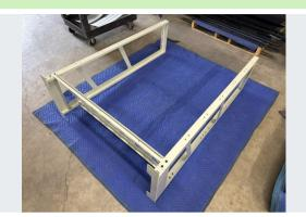
Install opposite side rack upright into existing shelf/upright assembly, install bolts and nuts, leaving them slightly snug.
