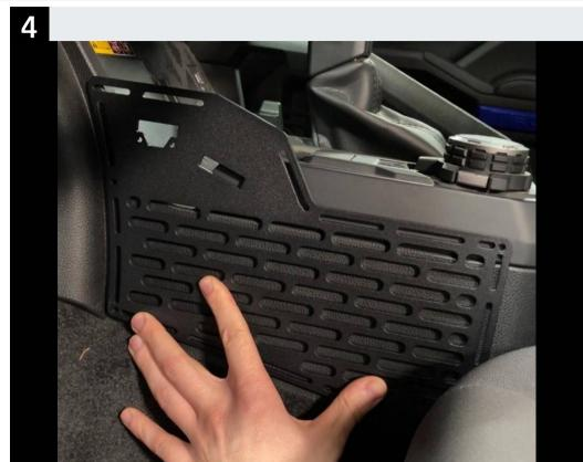
Install the stainless logo plate in both panels using the 10-24 hardware.
