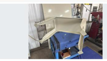
Roll the table onto its side to assist with the installation of the lower shelf.
