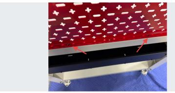
Fasten the panel to the table top through the two indicated holes using 2x 1/4" x 1/2" black button head screws, washers, and flange nuts.
