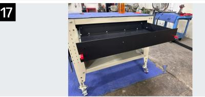
Set the drawer front onto the latches but do not install hardware yet.
