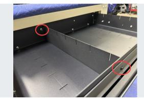
Use 2x 1/4" x 1/2" black button head screws, washers, and flange nuts to finish the divider installation.
