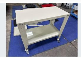
Set the table upright on a flat surface and ensure it is square. Then finish tightening the 3/8" nuts onto the carriage bolts.
