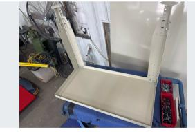
Invert the table top and attach the leg assemblies using the 3/8 carriage bolts, flange lock nuts and square-neck washers. The washers should be installed on the nut side.
