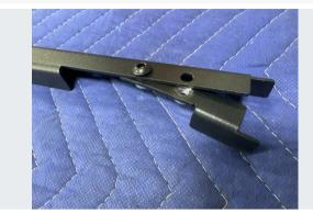
Pre-asseme the latch handle with  $1 \times 1/4$ "  $\times 3/8$ " black button head screws per side. Leave these slightly loose.
