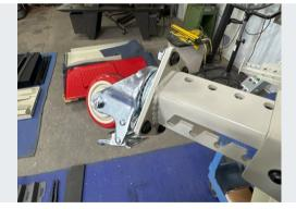
Secure casters with 5/16 x 5/8" button head screws, washers, and nuts; use 1/4 x 3/8" button head screws and washers for attaching feet.
