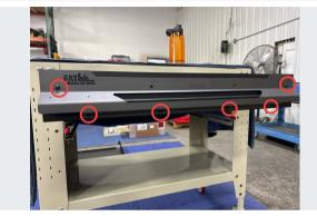
Install handle cover over handle using 6x 1/4" x 1/2" black button head screws, passing through the handle cover as well add the drawer front at the locations shown. Thread on flange nuts and tighten fully
