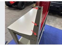
Attach each side of the Stack Rack panel to the mounting brackets using 3x 1/4" x 1/2" black button head screws, washers, and flange nuts.
