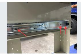
Install drawer slides into drawer mounts using 3x #10 x 1/2" button head screws and flange nuts. Slides will need to be partial extended to install the screw closest to the front of the table
