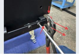
Slide handle assembly into latches with the "PRESS" cutout facing up, install but do not fully tighten the second 1/4" x 3/8" Black button head screw on each side, and center the assembly between the latches.
