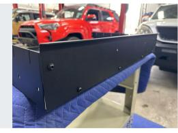
Install the drawer backyard panel onto the main drawer housing with 6x 1/4" x 1/2" button head screws, washers, and flange nuts.
