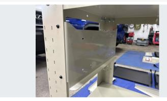
Install drawer mounts on each side using 4x 1/4" x 1/2" black button head screws and flange nuts per mount.
