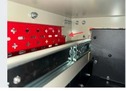
You may find access to the top mounting screws and nuts easier with the top drawer extended out all the way.
