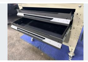
Repeat this process for the second drawer. Verify that drawers move smoothly without binding and that latches release and catchy properly.
