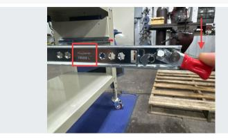
Slides indicate which side they should be installed on. Ensure that when installed, the latch lever actuates down to release the slide lock.
