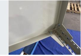
Attach the shelf to the legs at the lower mounting hole location using 8 more 3/8 carriage bolts, nuts, and square neck washers.
