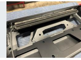
Install lightbar and adjust brackets so that the bar is centered in the opening. Tighten all of the mounting hardware for the bezel, brackets, and lightbar
