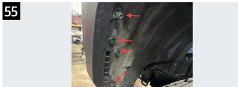
Fasten inside of flare to inner fender with (1) coarse thread screw and (3) plastic push retainers as shown.
