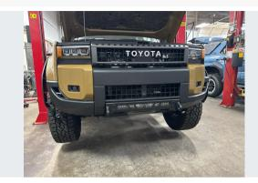
Temporarily reinstall the fascia assembly and take not of any areas that need to be trimmed or corrected, as well as any adjustments that the bumper may require.
