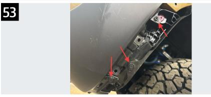
Continue reattaching the inner feeder to the lower fascia filler panel with another (2) plastic push retainers and (1) coarse thread screw.
