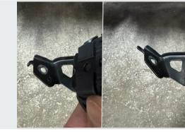
Flatten out the indexing tab on the horn mounting bracket.
