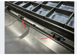
Release the tabs retaining the top filler panel along the top edge. There are (6)
