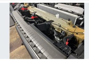
Reinstall and tighten upper grill mounting screws.
