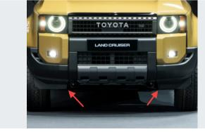
Remove front lower valance, if equipped. This will not be reinstalled
