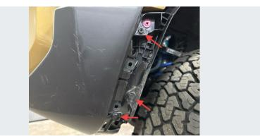
Remove (2) remaining clips and (1) screw beneath the flare.
