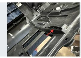
Depress the tab to release the retainer on both outer lower corners of the filler panel.
