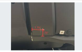
Mark the center grill surround pieces as shown in the diagram. Drill through the outer and inner layers of plastic with a 9/32" drill.
