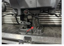
Thread the harness up through the facts reinforcement structure and the intercooler shroud. Snap the wire retainer into the unused slot on the latch mount support.
