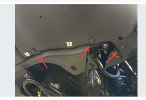
Remove (2) clips and (1) screw retaining the bottom of each of the lower fascia corner panels.
