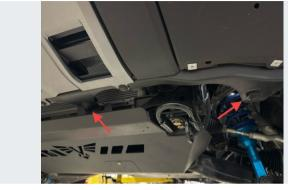
Remove (4) lower fascia retaining screws. There are (2) on each side.
