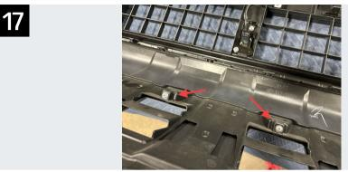
Remove the (2) Phillips screws in the center of the filler panel.
