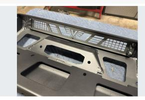
Install lightbar bezel and lightbar mounting brackets to the inside of the bumper using (4) 1/4" x 3/4" black button head screws, finish washers, and flange lock nuts.
