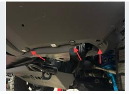
Reattach lower corner fascia panel to inner fender liner with (2) plastic push retainers and (1) coarse thread screw.
