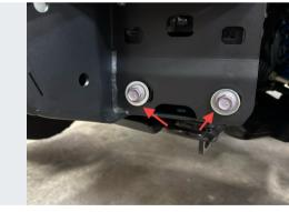
Attach the bumper to the mounts by reusing (2) of the original crash bar bolts per side, with the addition of a 1/2" USS washer on each bolt.
