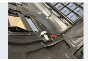
Remove the (2) white clips retaining the filler panel (1 on each side)
