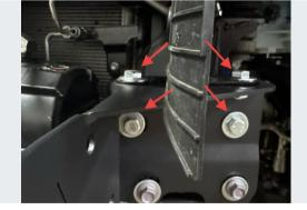
Using (1) 1/2" x 1" hex head screw, 1/2" USS washer, and 1/2" flange nut per mounting slot, attach the bumper to the remaining (4) mounting points on each side.
