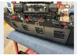
Remove the (4) clips retaining the bottom of the center fascia filler panel.
