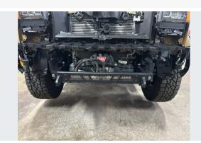
Install bumper into factory mounting flanges on the frame.
