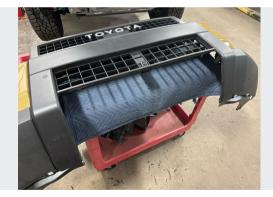
The cut fascia should look like this when completed. Clean up the cut edges with a flat disc or similar tool.
