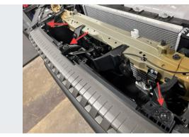
Remove the (3) grill mounting screws and set aside.
