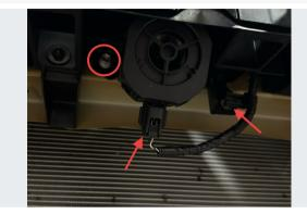
Disconnect the wire connector from the horn, and pop the plastic wire retainer out of its bracket. Remove the retaining bolt and remove the horn.
