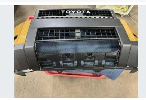
Prepare for the cut: using a stable surface such as a small work table or sturdy shop cart, flip the fascia over so that the outside is facing up.
