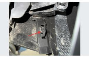
Depress center finger to release tab retainer on the inside bottom of the flare on each side.
