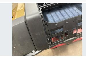
Using the channels the filler panel fit into previously as a guide, mark the fascia with a paint pen or similar.
