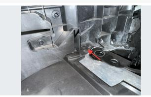
Remove the clip on each side fastening the side radiator shrouds to the crash support on both sides.
