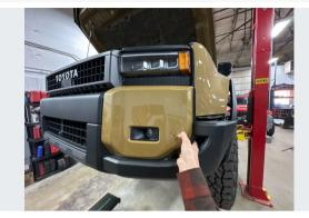
To remove fascia, use the vents in each side to carefully detach internal retainers and release the fascia one side at a time.
