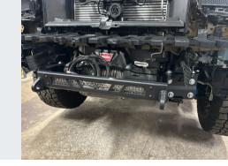
Once the the trimming is satisfactory and the fit of the bumper is even and correct, proceed in fully tightening all bumper mounting hardware on each side.
