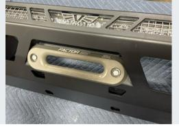
Install fairlead or fairlead block-off plate and tighten hardware
