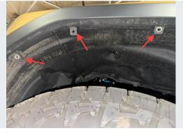
Reattach upper portion of fender flare with (3) plastic push retainers at indicated locations.
