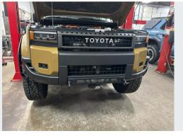
Reinstall front fascia assembly and snap the panels beneath the headlights back in place.
