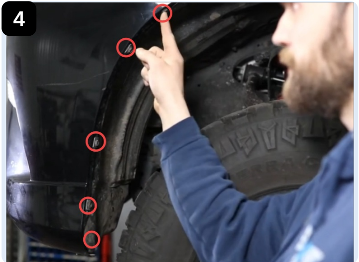
Remove the clips and screws retaining the front half of the inner fender liner.
