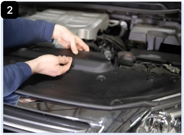
Begin by removing the clips retaining the upper radiator cover. Set the cover aside
