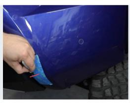
Measure down, holding the tape vertically across the fascia, and make a mark on the tape at 8-3/4".
