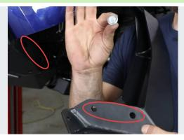
Begin by attaching the wings to the side flange of the bumper using the the holes on the internal flange of the wing with (2) 3/8-16 x 3/4" hex head cap screws, flat washers, and 3/8" flange lock nuts front of the wing to the bumper. Leave these slightly loose. per side. Leave these fasteners slightly loose.
