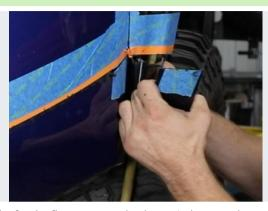
The marked portion of the fender flare may need to be entirely cut and removed before the portion of the fascia behind is accessible enough to cut all the way through.
