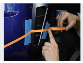
In similar fashion, use the fine-line tape to connect the second and third points to create a straight line across the remaining unmarked portion of the fascia, as well as the fender flare.
