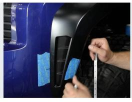
Apply another strip of masking tape along the fender flare tangent to the wheel opening, directly below the measurement starting point.
