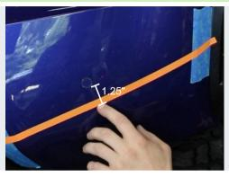
As a point of reference: the bottom profile of the parking sensor to the edge of the tape being used to indicate the cut-line should measure around 1-1/4" to 1-3/8" as shown in the image.
