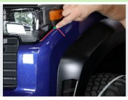
The second point will be measured starting from the convergent point of the fender-to-fascia seam, and the bottom edge of the headlight.
