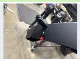
Once the wing is tight, install the rubber bumpers into the large hole of the fascia support brackets, and mount the bracket to the wing with (1) 1/4-20 x 3/4" black button-head socket cap screw on each side. Assist the bracket in the slot so that the bumper engages the inside of the fascia, providing gentle outward support.
