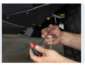
Tighten all wing hardware using a 7/32" hex and 9/16" socket and wrench. Start with the front outside hardware and work around to the inside hex heads. Check the fit of the wing as you go.
