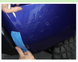
For the first point, begin by applying a strip of masking tape along the side of the Blitz bumper on the fascia.
