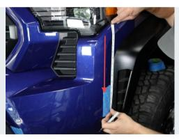
Once again using the flexible tape measure, allowing it fall vertically and follow the contour of the fascia, start from the point called out in the previous step and make a mark on the masking tape at 13.25".
