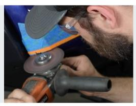
Take caution to avoid cutting the side of the Blitz bumper when to are closer to the center of the fascia.
