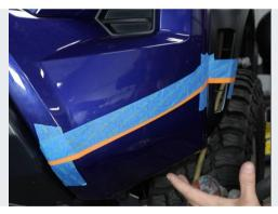
Before making the cut: it is advised to apply additional layers of tape to the fascia above the area being cut to help prevent and accidental damage.
