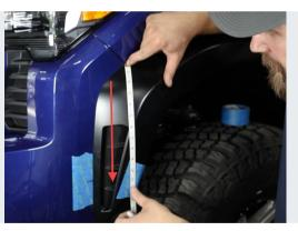
Again, allowing the flexible tape measure to fall vertically and hug the contour of the fender flare.
