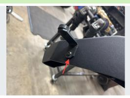
Once the wing is tight, install the rubber bumpers into the large hole of the fascia support brackets, and mount the bracket to the wing with (1) 1/4-20 x 3/4" black button-head socket cap screw on each side. Assist the bracket in the slot so that the bumper engages the inside of the fascia, providing gentle outward support.
