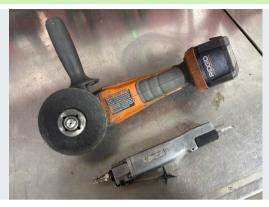
To make the cut you may use a small reciprocating saw or a cut-off tool with an abrasive disc. Always wear safety glasses and protective equipment when performing these operations.
