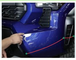
To make the cut will first require marking out three points on the bottom of the front fascia, along both sides.
