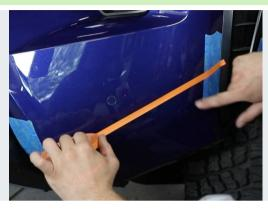
Using the edge of fine-line to follow the projection of the laser to create a cut-line, connect the two points.
