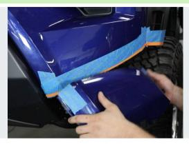
Once the cut is complete, remove the lower section of fascia and discard. Note: sometimes the plastic can slightly melt back together so this may require a slight snap to get it to separate, or the assistance of a utility knife.
