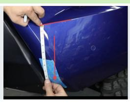
Using a flexible tape measure, hold the end flush with the sharp edge of the body line, right at the front point where it creates a shallow internal corner.
