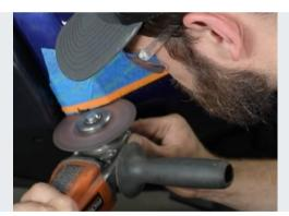
Take caution to avoid cutting the side of the Blitz bumper when to are closer to the center of the fascia.
