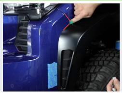
The third point will be measured from the intersection point of the fascia-fender seam and the outer profile of the fender flare where it crosses that sea, as indicated in the image.
