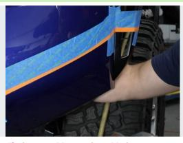
Additionally, be sure to verify that any wiring or other critical components are moved away from the backside of the cut or are well protected.
