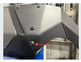
Install the remaining black 3/8-16 x 3/4" button-head socket cap screw and flange lock nut in the final mounting hole in the bottom of the bumper.
