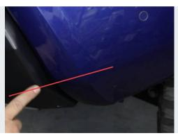
The cut being marked will be following closely in line with the bend in the front bumper just above the three Viper Wing mounting slots.
