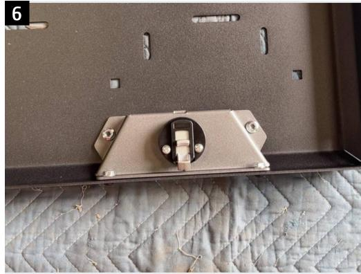
Mount the handle brackets onto the inside of the door using the provided 1/4"-20 x 1/2" button heads, and 1/4"-20 serrated flange nuts with a 1/4" washer under the head of each bolt.
