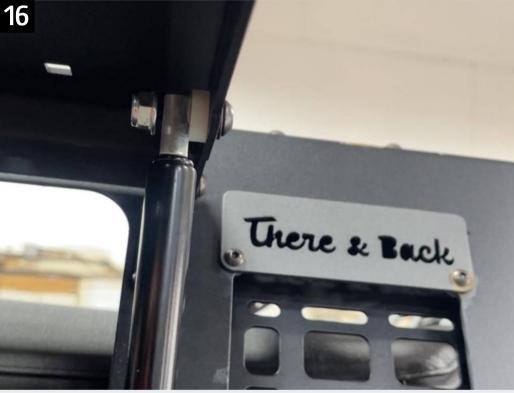
To get the plastic washer in place, a simple method is to rest the door on the hinge bracket and move it or hinge it enough to provide space to slide the washer into position. This way, it is possible to hold on to and adjust the washer while inserting the bolt through. Once the bolt is through the door and washer, maneuver the door until the bolt can pass through the hinge bracket as well.
