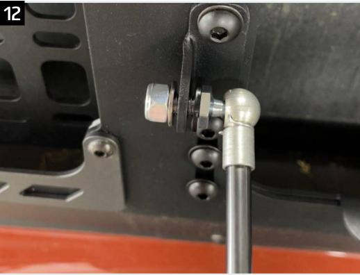
Mount the strut to its mounting bracket as shown. Make sure the knuckle end is on the outer side of the bracket. A plastic washer should be installed between the knuckle and the mounting bracket with an m8 washer and nylock nut on the other side. Tighten the nut using two 13mm wrenches.
