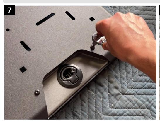
With all bolts loosely started, tighten the handle brackets into place.
