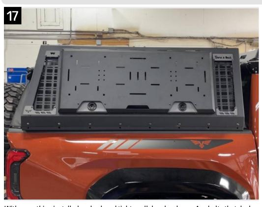
Note: Check that the door opens and closes as expected and that it latches properly. The latch bracket can be slid up in its slot as a form of adjustment if needed. Once everything is adjusted to your liking, your install is complete!
