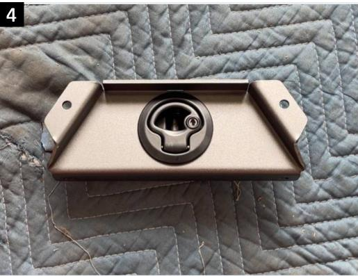
Begin by removing the backer plate from the latches with a Phillips screwdriver.
