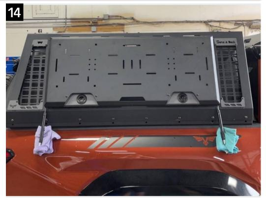
Install the door onto the hinge brackets. Use the 5/16"-18 x 1" bolts and 5/16" washers to pass through the hole in the door as well as the hole in the hinge bracket with a plastic washer sandwiched between the two and a 5/16"-18 flanged nylock nut on the inside. This step is easiest with the help of another person to ensure the door does not fall during the process. Do this on both sides.
