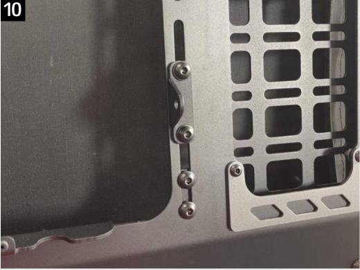
Mount the latch bracket to the inside of the bottom slot of the bed rack as shown using the 5/16"- $18 \times 3/4$ " button heads and 5/16" washer under the head of each bolt. With the bolts loosely started, slide the bracket all the way down in the slot and tighten all hardware.
