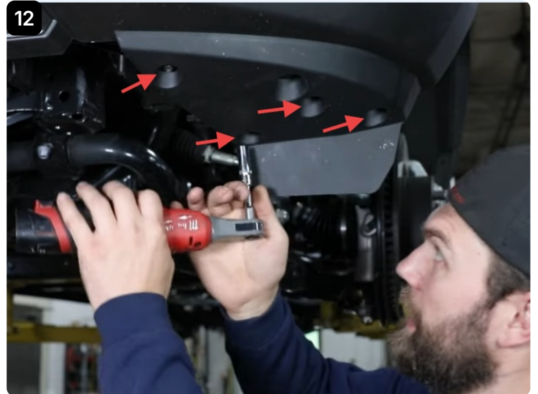
Remove (4) screws retaining the lower outer corner of the fascia.
