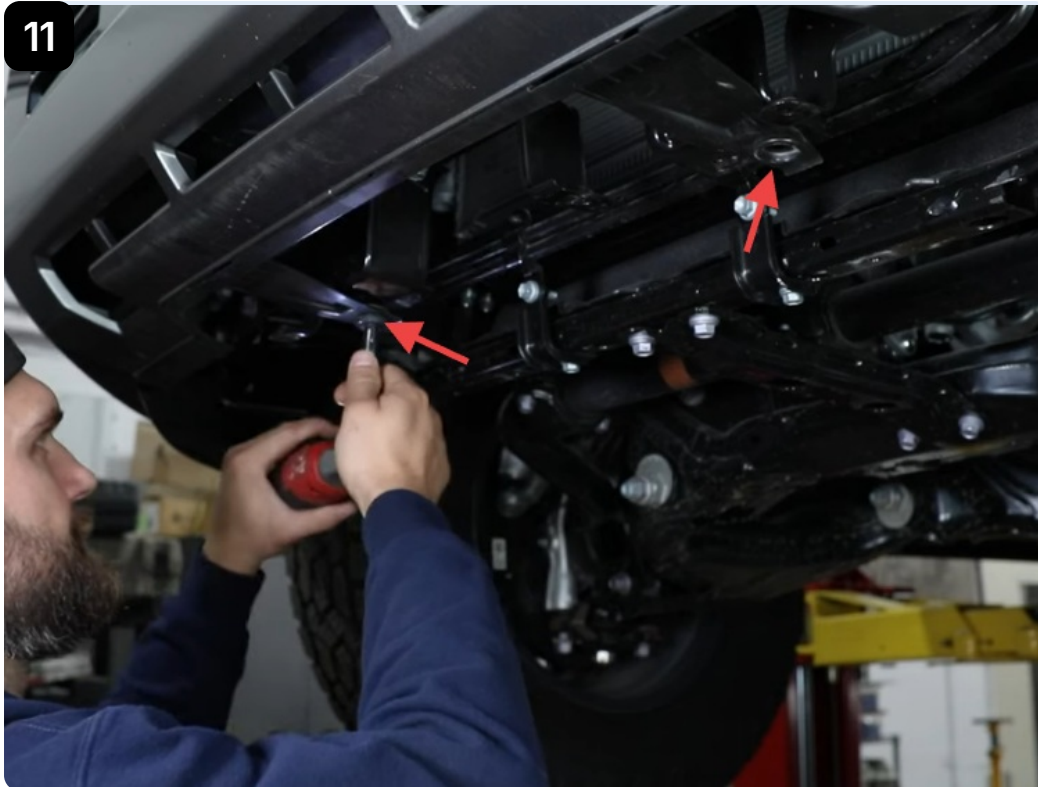
Remove the (2) rubber isolated fasters retaining the center of the fascia.
