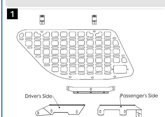
Included Parts: Molle panel | Upper Mounting Brackets | Lower Mounting Bracket | Driver's Side Hidden Mounting Bracket | Passenger's Side Hidden Mounting Bracket
