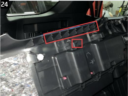
Remove the eight ribs boxed in the image above. This can be done using a razor blade. Try to cut them as close to the panel as possible to ensure fitment over the hidden bracket. At the same time, remove the plastic clip located in the other position boxed in the image above.
