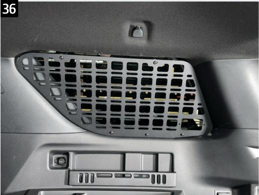
Hold the molle panel up the the mounting brackets and ensure that they are properly positioned before tightening the molle into place using the five smaller 1/4" bolts and nuts. If the panel is not sitting properly, adjust the mounting brackets prior to fully installing the panel.
