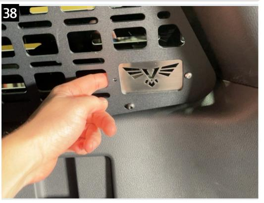
To complete the install, mount the logo plate to the molle panel between it and the window as shown. This can be done using the 10-24 bolts.
