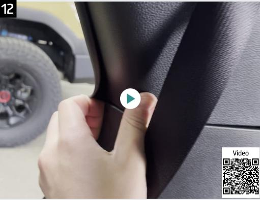
Begin moving up towards the front of the vehicle, prying out on the upper edge of the panel along the way.
