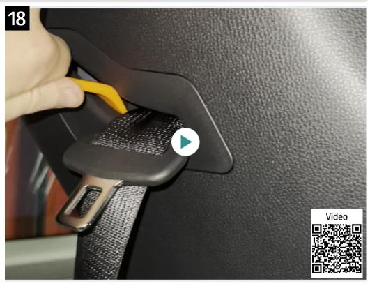
Pry out on the bottom of the plastic surrounding the seat belt to remove it from the larger panel.
