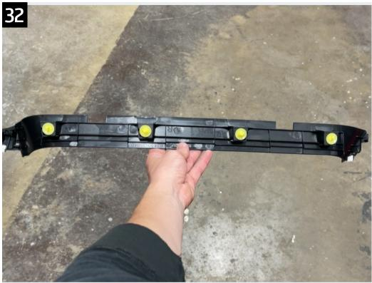
Pull the trim back out and cut out a rectangle to fit around the upper brackets. The back edge of the cut can be on the first rib in from the edge. This can be done using a razor blade.
