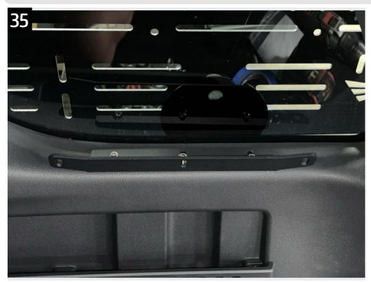
Install the lower mounting bracket into the hidden bracket, pinching the plastic between the two, using the three longer 1/4 bolts. Position it so it is parallel to the inner face of the plastic below it and tighten it into place. This may need to be adjusted later.
