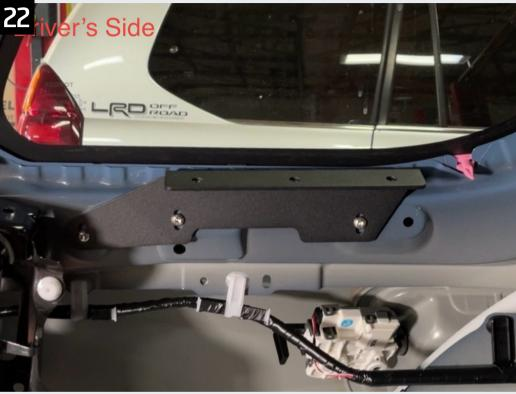
Install the hidden mounting bracket using three m6 button head bolts. Roughly center the front two bolts and tighten everything into place. This position may need to be adjusted later. Driver's side shown above. Passengers's side show in previous step.
