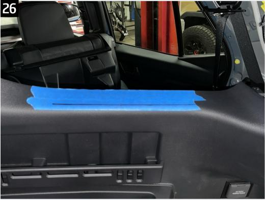
Pop the lower panel back into place and translate the previous measurement onto it. Make sure the top edge of the panel is where it normally sits before measuring off of the window in the same method used in the previous step.
