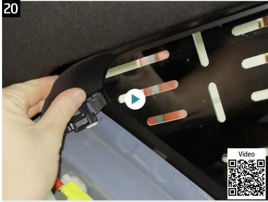
Pry out on the upper, front corner of the panel to pop it out of place. It may be helpful to Pry down on the front or rear edge the trim located above the rear window. As the clips pull out some of the trim in the door to allow for an easier time grabbing the edge of the panel. Once it is free, the seat belt and trim can be passed through the hole in the panel to get it out of the way entirely.
