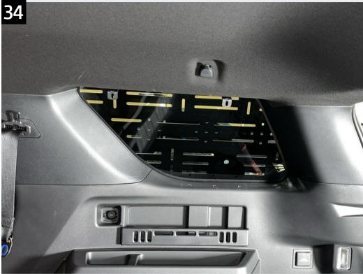
Pop all plastic pieces back into place in the reverse order they were pulled out. Be sure to plug in the wires that were disconnected during the disassembly at this time. Leave any bolts removed out for now.
