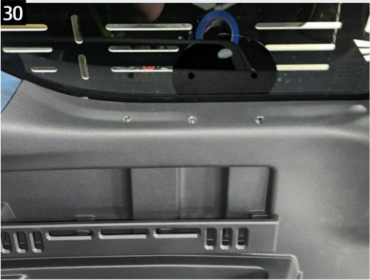
With the lines marked on the plastic, drill the three intersections out to fit a 1/4" bolt. Pop the plastic back into position to make sure the holes line up with the holes in the hidden bracket.
