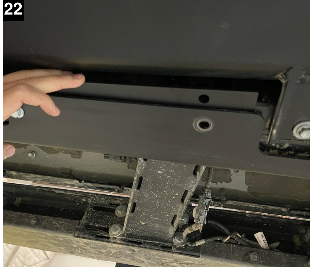
Slide the provided spacer in place between the frame and mount.
