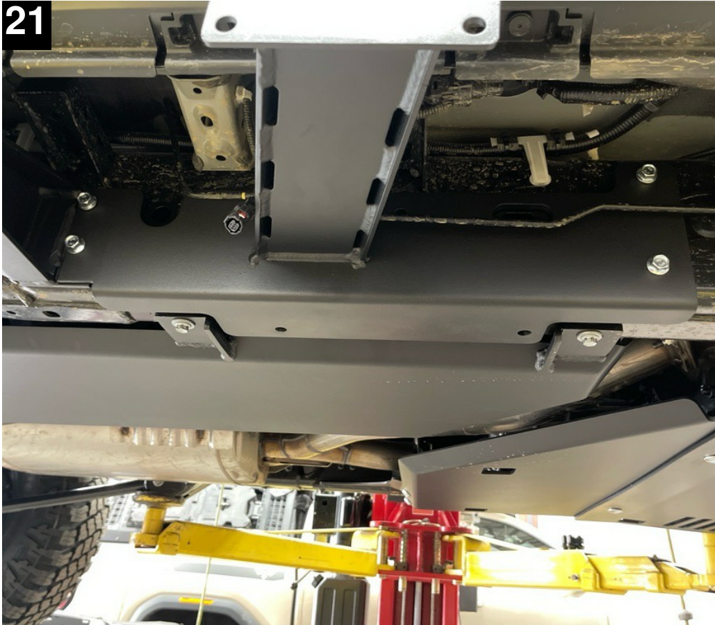
Loosely install the middle mount using the M10 bolts in the front and back. The back should mount over the front of the rear mount.
