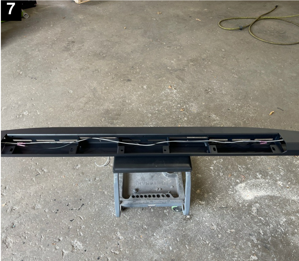
7 The wiring should look something like the image shown. Cover each connector with heat shrink or electrical tape.
