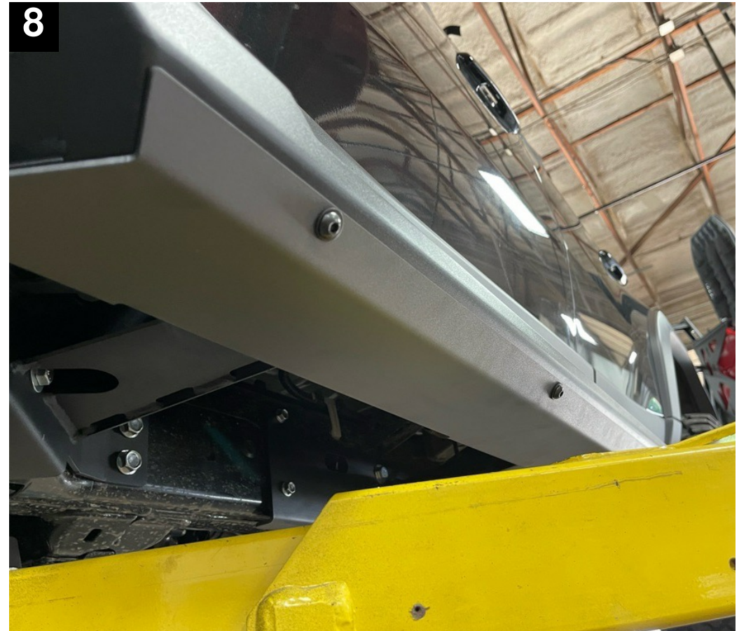
8 Bolt the skid plate onto the bottom of the slider using the 5/16" button heads and washers washers and flange nuts.
