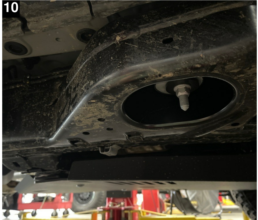
10 Remove the plastic panel underneath the body mount. To do this, use something like a screw driver to push up and in on the two recessed tabs while pulling down on the panel.
