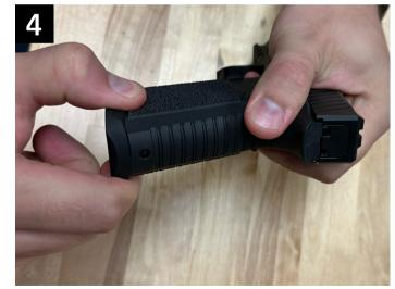
To test correct installation pull SCT 19 Magwell in opposite direction from frame. Magwell should not come out.
