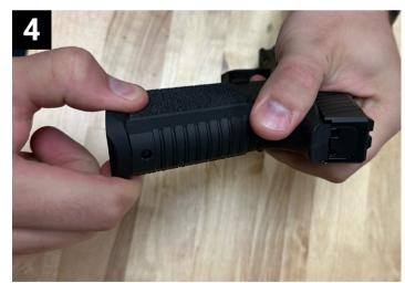
To test correct installation pull SCT 19 Magwell in opposite direction from frame. Magwell should not come out.
