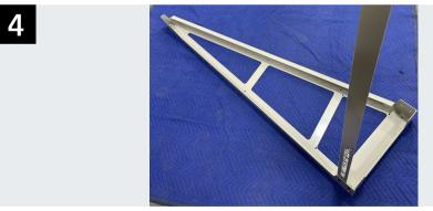
Begin with one of the rack uprights laying on its side, with the "open" side of the upright facing up. Attach one lateral brace to the lower back mount points with the supplied 5/16" button head screws and flange lock nuts. Snug but do not tighten these fasteners.
