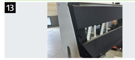
Install each punch rack onto the frame with 4 5/16 hex head screws, washers, and flange lock nuts.
