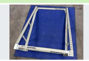
Roll the assembly over so that the lateral brace is supporting the upright, and the slotted face of the upright is facing up. Attach the opposite side rack upright to the other end of the lateral brace. Snug this hardware.
