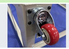
Install casters on the bottom of both rack uprights using 5/16" button head screws and 5/16" flange Lock the casters and stand the rack up. lock nuts. Tighten these fully.
