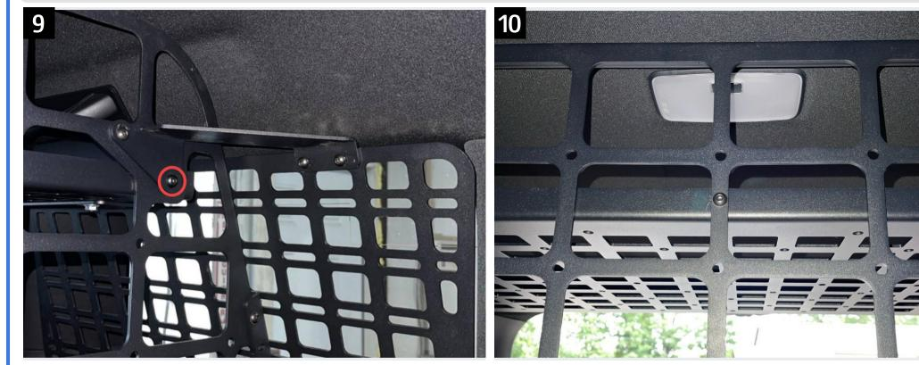
Loosely install the upper mounting bracket. If installing with an upper shelf, the lower bolt will go through that as well in the location circled in red. This will require the longer 1/4" bolt provided with the upper shelf. Doing this may require moving the panel or basket forward or backward. If installing with an upper shelf, secure the center of the panel to the shelf with 1/4" hardware.
