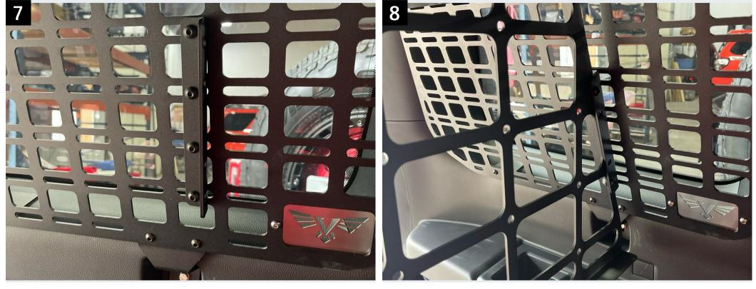
Loosely install the lower mounting brackets on each side. It should be mounted in the slots above the front mounting hole of the lower molle panel mount. This bracket can be flipped upside down depending on how far forward or backward you want the panel to sit.
