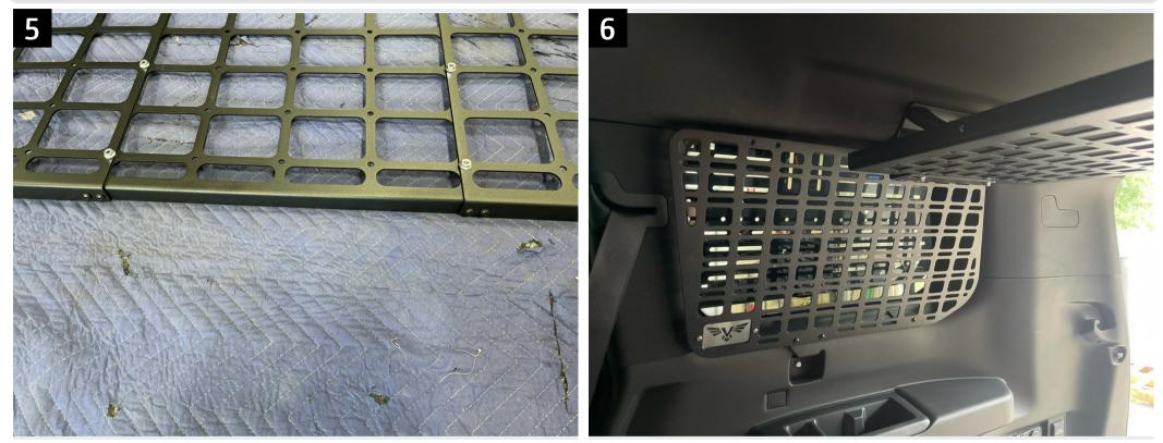
Repeat the previous step on the bottom flange. The nuts should go on the top of the flange. Once all bolts are installed, they can be tightened.
