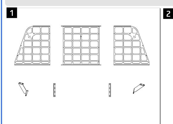
Included Parts: Pet divider side sections | center section | upper and lower mounts.
