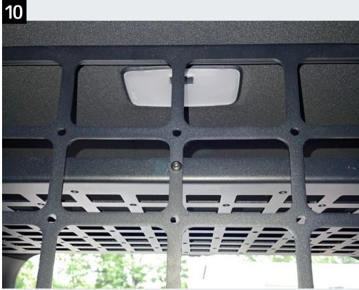
Loosely install the upper mounting bracket. The hole circled in the image will need to be the longer 1/4" bolt provided. If installing with an upper shelf, the lower bolt will go through that as well. Doing this may require moving the panel or basket forward or backward.
