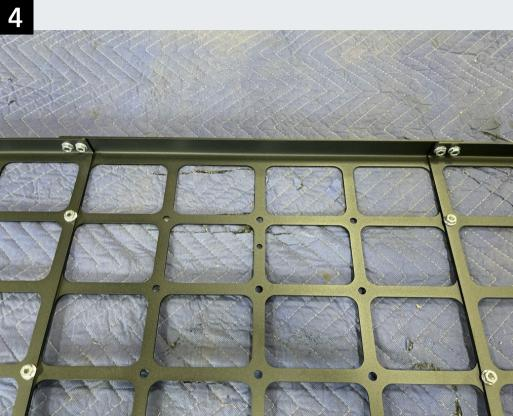
Begin by bolting the panels together through the vertical face using the provided 1/4" hardware. It is best for the nuts to be on the face that will point towards the rear of the vehicle.
