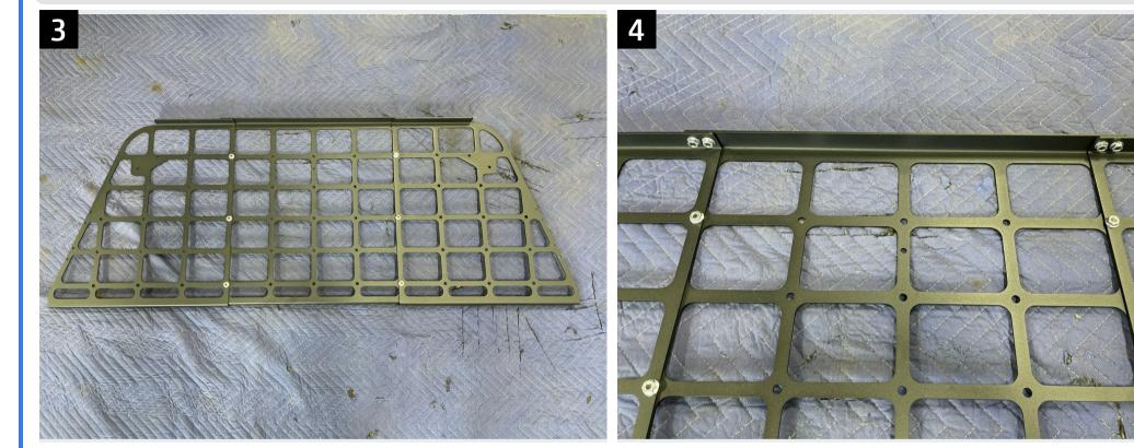
Begin by bolting the panels together through the vertical face using the provided 1/4" hardware. It is best for the nuts to be on the face that will point towards the rear of the vehicle.
