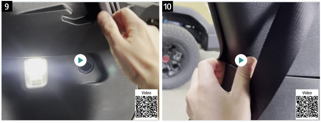
Begin moving up towards the front of the vehicle, prying out on the upper edge of the panel along the way.
