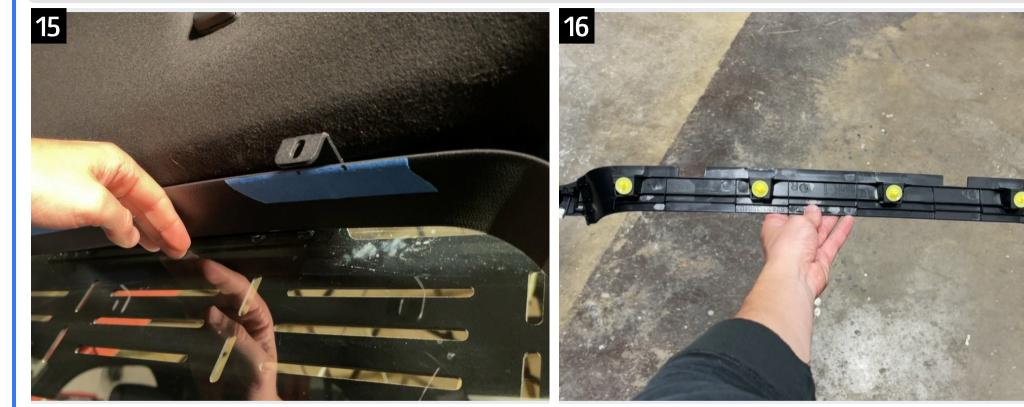
Put the upper trim roughly into position over the mounting brackets and mark outside of the edges of each to indicated where to make a cut.
