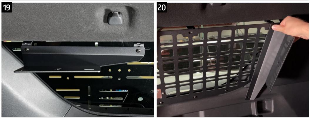
Install the shelf mounts onto the upper mounting brackets using the longer 1/4" bolts, washers and nuts as shown. Position the mounts as desired and tighten them into place. Make sure the arrow cut into each is pointing towards the front of the vehicle.
