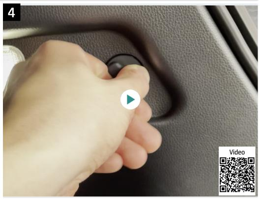
Begin by removing the net hook by twisting it clockwise and pulling out to reveal the bolt behind it.
