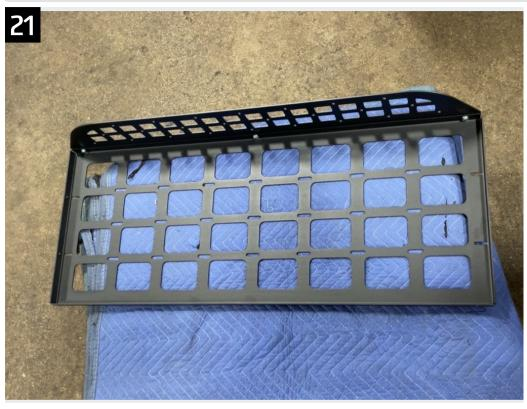
Install the front panel onto one side of the shelf using the shorter 1/4" bolts, washers and nuts.
