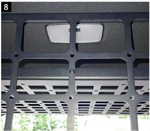
If installing with a pet divider, secure the center of the panel to the shelf with 1/4" hardware.
