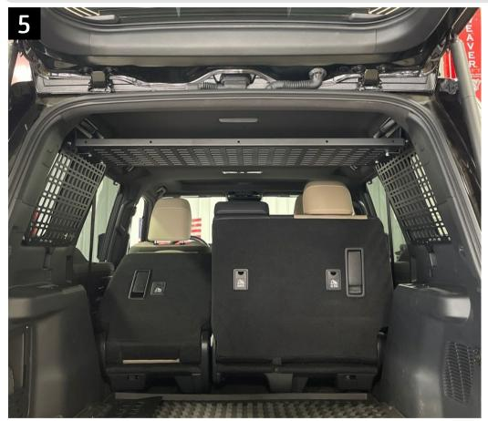
Place the shelf onto the mounting brackets and loosely secure it using the short 1/4" hardware.
