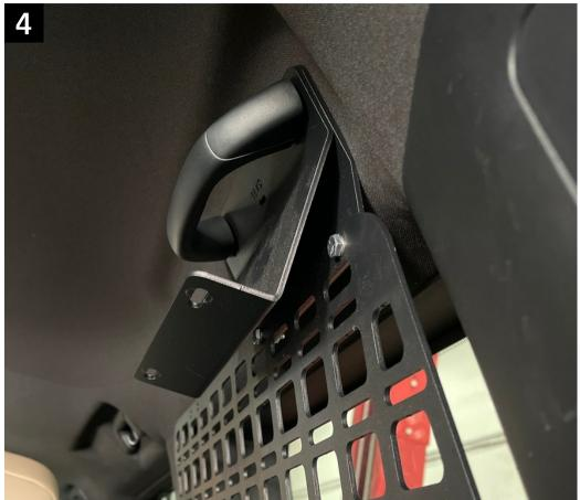
Install the mounting brackets with the handle mounting holes and the factory hardware. This can be installed with or without the handles. If installing with the rear window molle panels, stack the shelf mounting bracket over the molle panel mounting bracket. Longer M6 bolts and small washers are provided if the stack up for your set up is too much for the factory hardware.
