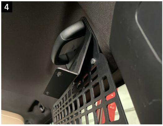
Install the mounting brackets with the handle mounting holes and the factory hardware. This can be installed with or without the handles. If installing with the rear window molle panels, stack the shelf mounting bracket over the molle panel mounting bracket. Longer M6 bolts and small washers are provided if the stack up for your set up is too much for the factory hardware.
