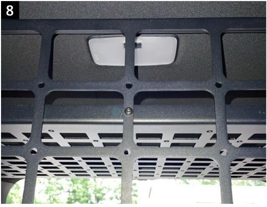
If installing with a pet divider, secure the center of the panel to the shelf with 1/4" hardware.
