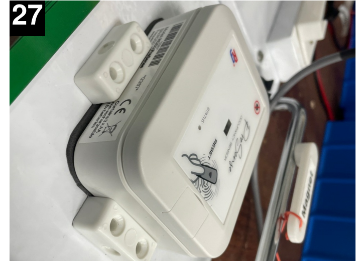
27 Place box in fixture in orientation shown, with barcode facing you and cover as photo
