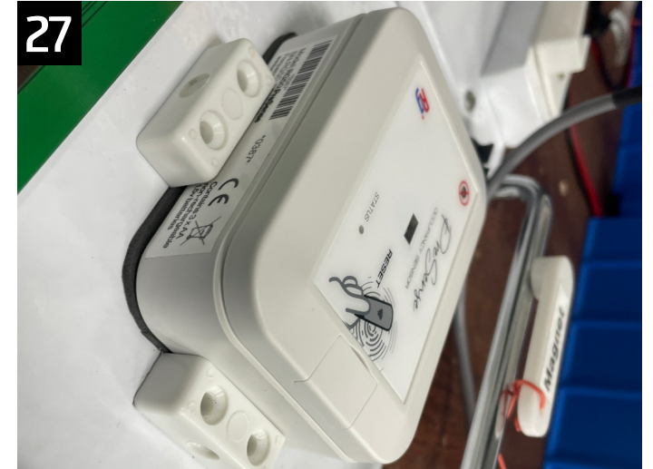
27 Place box in fixture in orientation shown, with barcode facing you and cover as photo
