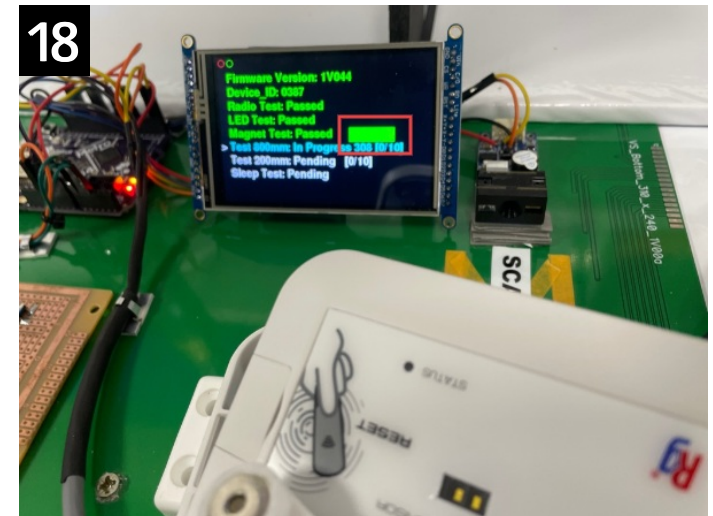
18 Hold magnet to reader and look for green bar on screen to indicate pass. If green bar then HIT TEST PASSED
