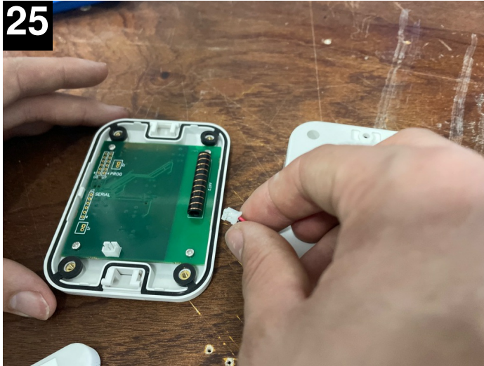
25 Remove cable for 3 seconds to reset unit
