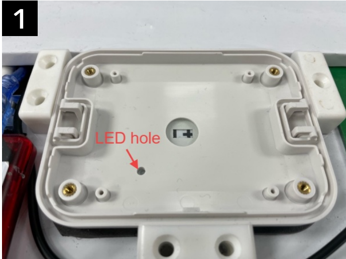
1 Take front cover and place on fixture as shown. Ensure LED HOLE is bottom half!
