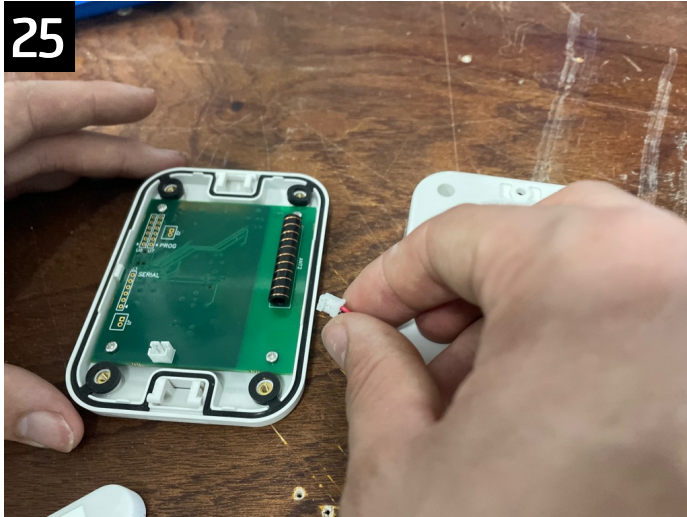
25 Remove cable for 3 seconds to reset unit
