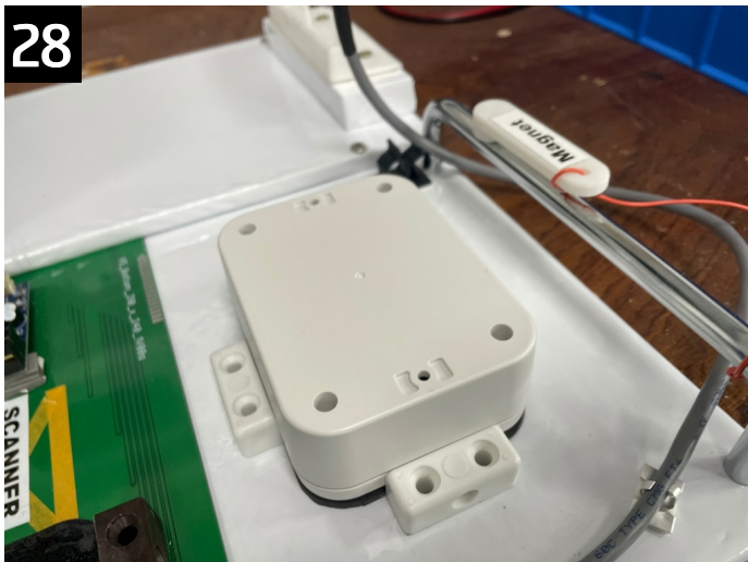
28 Flip over box and insert x4 screws
