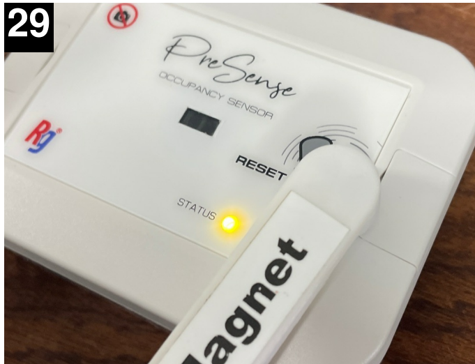
29 blue LED stops (30 secs) place magnet for 10 secs until solid YELLOW GOES OUT. White LED will flash each 10 to confirm
