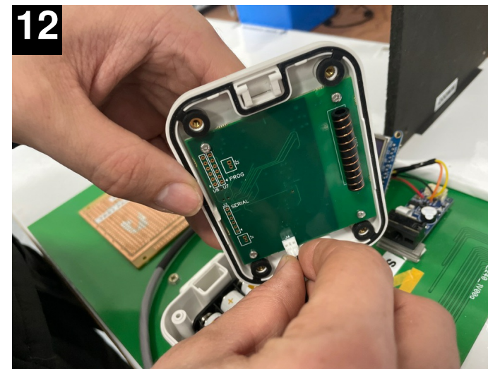
12 Connect battery connector from back cover to PCB.
