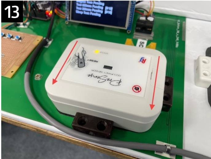
13 Place front cover on to back cover. It will look UPSIDE DOWN to you.
