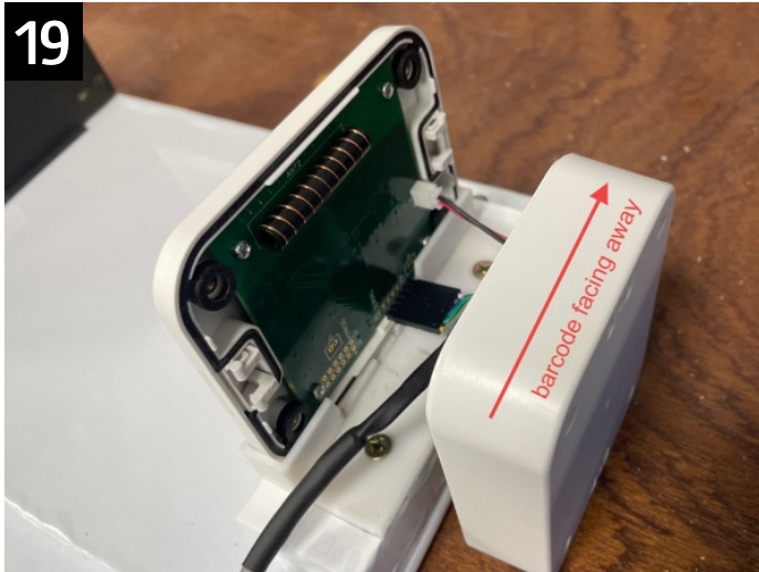
Place in test fixture - BARCODE FACING AWAY FROM YOU
