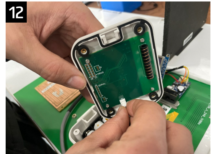
12 Connect battery connector from back cover to PCB.
