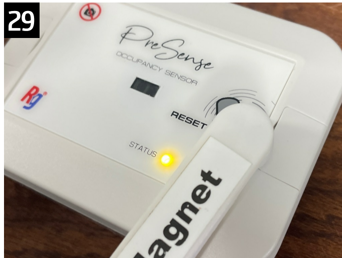
29 blue LED stops (30 secs) place magnet for 10 secs until solid YELLOW GOES OUT. White LED will flash each 10 to confirm
