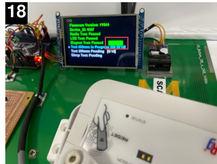
Hold magnet to reader and look for green bar on screen to indicate pass. If green bar then HIT TEST PASSED
