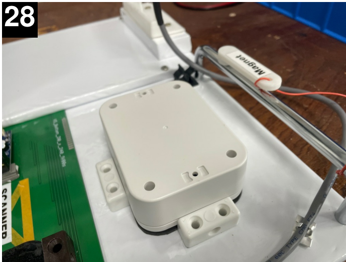
28 Flip over box and insert x4 screws
