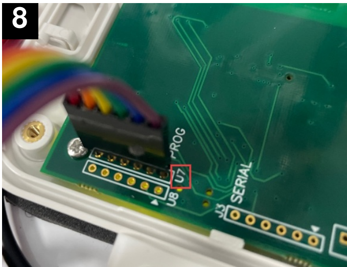
8 Insert programming cable into U7
