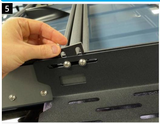
With the hardware still loose, slide the slotted aluminum spacers in between the side rail and bracket from the top. \*These spacers will only be used when the rack is equipped with gray side accent panels.\*
