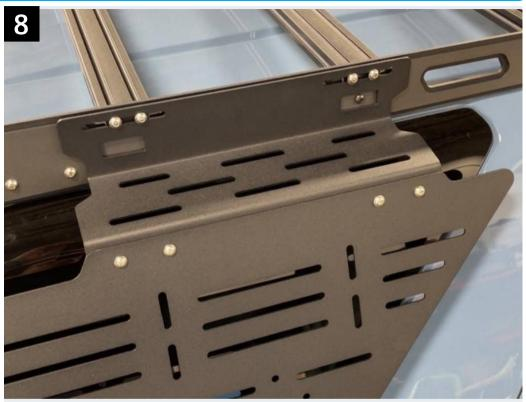
Attach the accessory panel to the outside of the mounting bracket using the (4) 1/4x20x3/4" bolts washers and serrated nuts.
