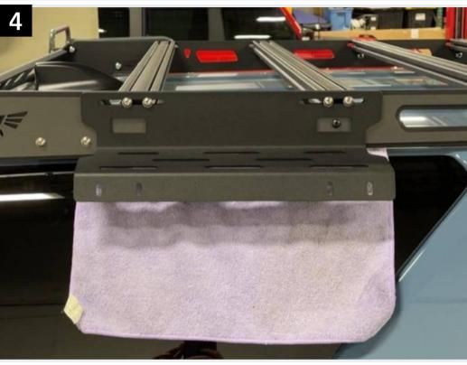
Loosely install upper mounting bracket using the 1/4x20x1" bolts with washers
