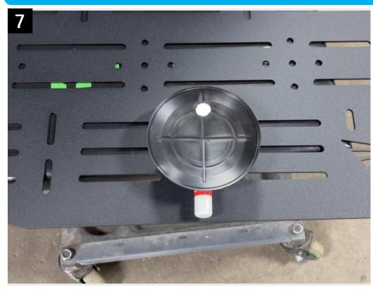
Orient the suction cup as show with the pump button down and tighten with a 5/32" allen.
