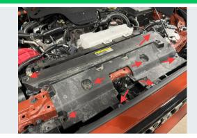
Remove the (8) plastic retainers holding the radiator cover, and set aside cover.
