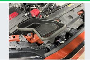
Reinstall air intake extension and fasten down with plastic push clips removed during disassembly.
