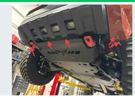
From the underside, remove fasteners retaining the lower fascia to the crash support and inner structure. This may vary depending on your trim level.
