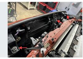
Reinstall the upper grill mount fasteners and tighten.
