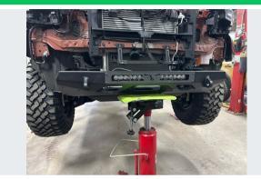
Using a jack or the assistance of a friend, lift the bumper into place, ensuring the mounts are lining up and the posts on the frame mounts pass through the windows on each bumper mount.
