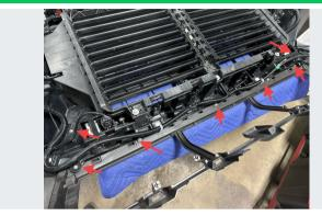
Remove the (7) Phillips screws retaining the center fascia filler panel.
