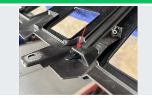
Working around the perimeter of the lower filler panel, depress the tongue of the retainers one at a time while gently separating the filler panel from the fascia until the panel comes free from the fascia.
