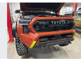
Reinstall the front fascia assembly over the bumper, taking care not to scrape the sides of the fascia against the outside of the flares. An extra set of hands will make this process much easier.
