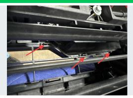
Gently press the the filler panel into place, ensuring all of the retention tabs engage correctly and snap securely into place.
