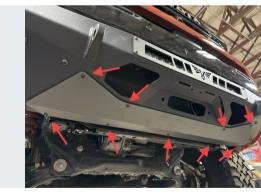
Install the included lower skid to the bottom of the bumper using the retaining (9) 1/4-20 x 3/4" black button head screws and 1/4" flange nuts.
