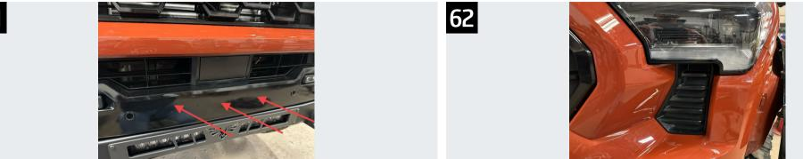
With the fascia hanging on the core support apply pressure to the center to ensure the three internal Verify that the fascia is nested around the headlights correctly on both sides. retainers are clicked into place.
