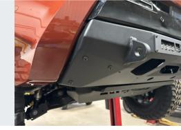
Use (3) black 3/8-16 x 3/4" button head screws and 3/8-16 flange lock nuts to close off Viper Wing mounting slots.
