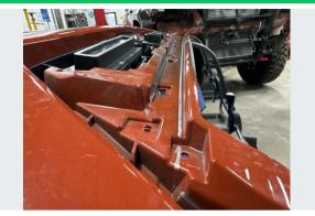
Mark a line across the center of the fascia, offset approximately 1/8" above the lip, below the row of filler panel mounting tab slots.
