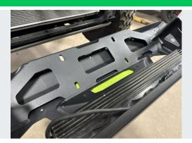
If you are installing a winch, now is the time to do that as well using the hardware supplied with your winch. **Tighten fully before installing on the truck.**If you are installing a larger winch, slide as far back as possible before installing skid plate.
