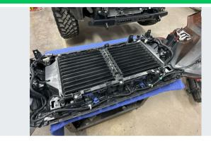
Remove the fascia assembly one final time and set upside down on a blanket or other non-scratch surface.
