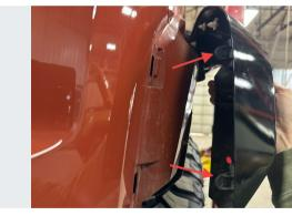
Un-snap fender flares from fascia by depressing tongue on retainers from inside of the fascia, accessed through the inner fender. Pop additional retainers out from the fender by gently pulling outward.
