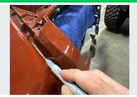
Using the relief for the lower filler panel along each side of the center fascia opening as a guide, mark a cut line approximately 1/4" away from the lower surface of the relief channel.
