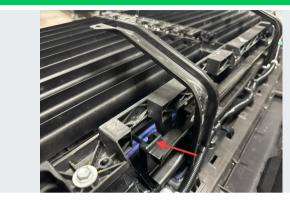
Carefully lift the tab on the (3) lower fascia mounting bracket retainers and remove the mounting bracket as an assembly.
