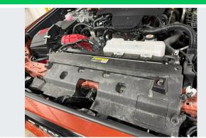
Reinstall upper radiator shroud and fasten with plastic push clips removed during disassembly.
