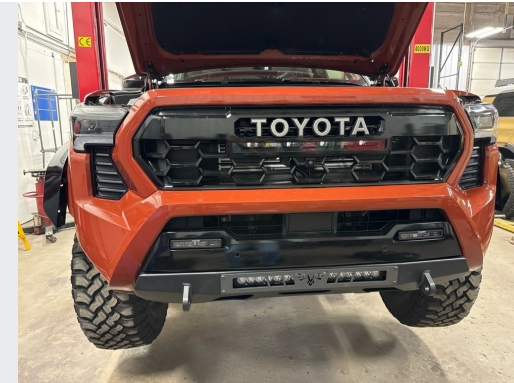
For the final time, reinstall the front fascia assembly and begin fastening it to the truck.
