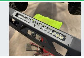
Install thelightbar bezel into the front face of the bumper using (4) 1/4-20 x 3/4" black button head screws, 1/4-20 flame lock nuts, and tighten with a 5/32" hex.
