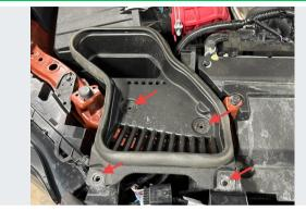
Remove the (4) fasteners retaining the intake shroud, as well as the shroud itself.
