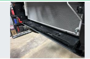
Remove the plastic lower radiator splash guard. There are (9) plastic clips retaining it to the chassis. (3) in
