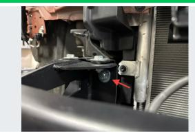
Install the remaining (2) 7/16 hex cap screws, flat washers, and nuts through the remaining non-threaded mounting hole in the frame mounts.
