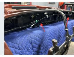
Before making the cut, ensure that all wire harnesses and important sensors are protected and out of the way of the cut.
