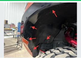
Remove fasteners retaining forward half of fender flares, as well as fasteners retaining the front of the inner fender liners. This may vary depending on your trim level.
