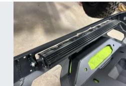
If you are installing a lightbar, now is the time to do that using the welded-in mounting provisions. Spacers may need to be used to center the lightbar and take up any excess space between the mounts.
