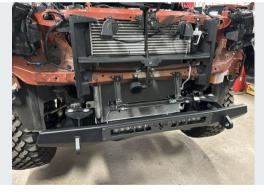
With the bumper alignment determined and the fascia assembly still removed, tighten the bumper to the truck.
