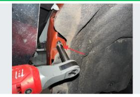
Reinstall and tighten the fastener that was removed from the inner lip of the fascia just below the retainer at the fender.
