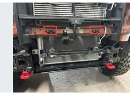
Reinstall the lower fascia mounting bracket onto the core support, re-using the factory hardware.
