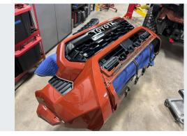
**Prepare for the cut:** using a stable surface such as a small work table or sturdy shop cart, flip the fascia over so that the outside is facing up.
