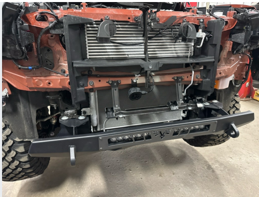
With the bumper alignment determined and the fascia assembly still removed, tighten the bumper to the truck.
