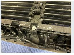
If additional space for the control box is required, such as with the updated new Zeon, the lower shutter mounting bracket may need clearanced.
