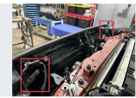
Disconnect fascia harness. There are (2) connectors on both sides of the grill shell, totaling (4) connectors.
