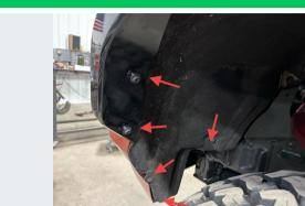
Reinstall and tighten inner fender and fever flare coarse-thread fasteners.
