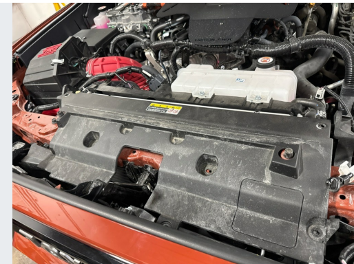
Reinstall upper radiator shroud and fasten with plastic push clips removed during disassembly.
