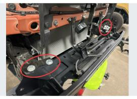
Using (4) 7/16-14 x 1" hex cap screws, (4) flat washers, and (4) 7/16-14 flame lock nuts, attach the bumper to the frame mounts at the four top mounting points.
