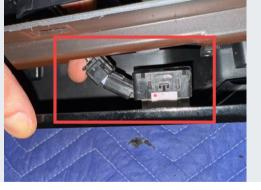
Detach the remaining (2) plastic tabs retaining the center filler panel and separate the panel from the fascia.
