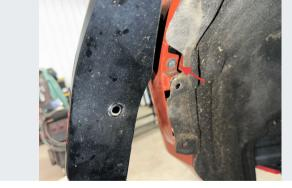
Remove screws retaining the fascia at the wheel opening. These are a 10mm hex.
