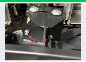
Re-using (4) of the factory crash bar mounting bolts (2 per side) install them into the factory threaded mounting points through the remaining bumper mounting slots on the lower portion of the mounts.
