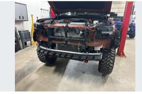
At this point you may carefully remove the entire fascia as an assembly. Gently lifting the fascia as you pull away from the front of the truck with aid in removal. This will be made easier with an addition person to help avoid dropping the fascia assembly.
