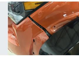
Gently pull outwards to disconnect fascia from internal retention bracket on each side.
