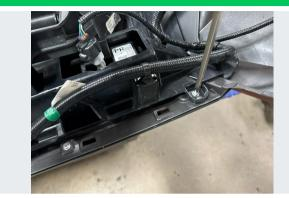
Reinstall Phillips screws, and tighten.
