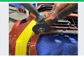
Cut the center of the fascia out using the marked out tape lines as a guide, taking caution to avoid contacting the visible portions of the fascia.
