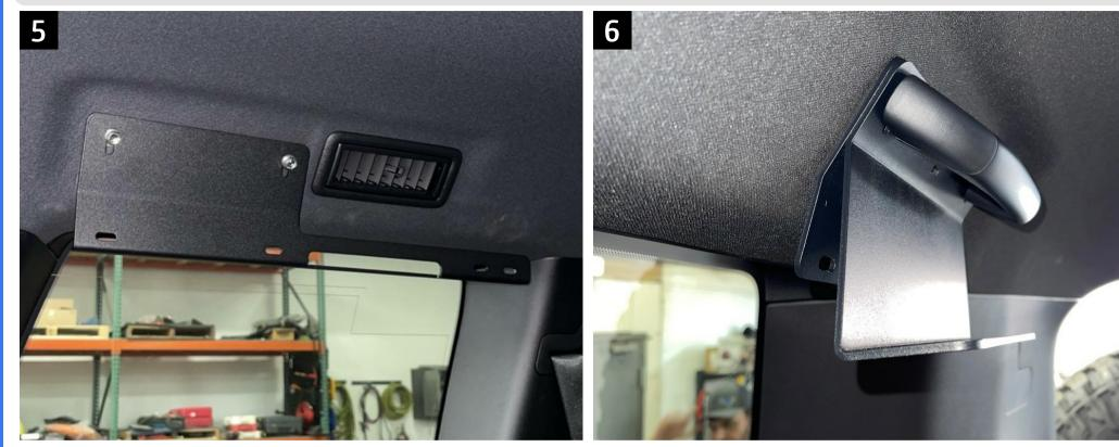
Now take the provided upper bracket and bolt them into the factory holes that held the handle into place, using the factory hardware. The handles can be installed over the shown. Longer M6 hardware is provided if extra thread engagement is needed for your brackets or left off. Install as shown in the orientation above. Leave this loose for now for adjustment.
