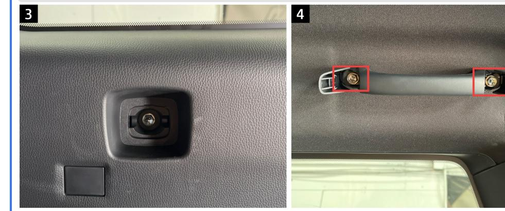
Start by removing the plastic cover, below the rear window, with a pry tool or a flat head screw driver. Once removed, use a 10mm socket to remove the hex bolt. Be sure to hold onto this for later use. Next, you need to remove the grab handles from each side of the vehicle. Pop off the plastic covers and remove the (2) factory hex bolts using a 10mm socket. Repeat this on each side of the vehicle.
