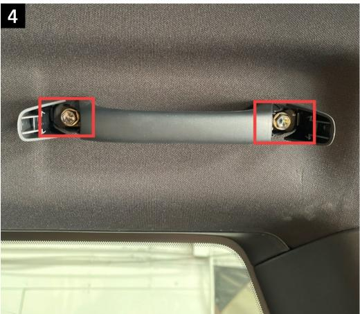
Next, you need to remove the grab handles from each side of the vehicle. Pop off the plastic covers and remove the (2) factory hex bolts using a 10mm socket. Repeat this on each side of the vehicle.
