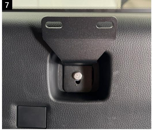
Take the provided lower bracket and bolt it into place in the orientation shown above, using the provided long m6 bolt and spacer behind the bracket. Leave this loose for now so you can have adjustment if needed.
