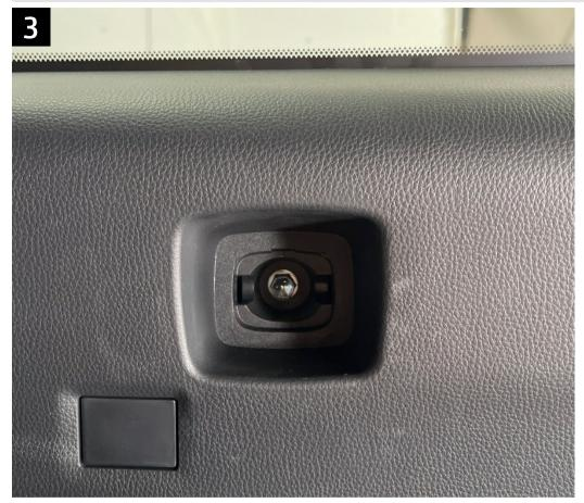
Start by removing the plastic cover, below the rear window, with a pry tool or a flat head screw driver. Once removed, use a 10mm socket to remove the hex bolt. Be sure to hold onto this for later use.
