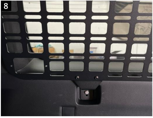
With your brackets loosely bolted into place, bolt your molle panel to the lower bracket using the provided 1/4" button heads and a flange nuts.
