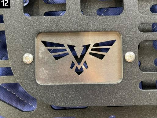
Take the provided double sided 3M tape and cut to size of the last remaining brackets. Once cut to size peel one side of the tape off and place on the bottom side of the bracket, as shown above. Peel the other side of the tape, and feed the bracket through the logo hole and shimmy down to the mounting hole on the bracket and stick to the plastic and bolt into place.
