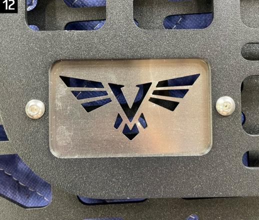
Take the provided double sided 3M tape and cut to size of the last remaining brackets. Once cut to size peel one side of the tape off and place on the bottom side of the bracket, as shown above. Peel the other side of the tape, and feed the bracket through the logo hole and shimmy down to the mounting hole on the bracket and stick to the plastic and bolt into place.
