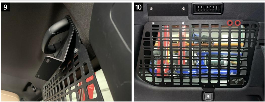
Next, take the provided 1/4" hex heads with a washer and flange nut and bolt them to the top back bracket as shown above using a 7/16" wrench.
