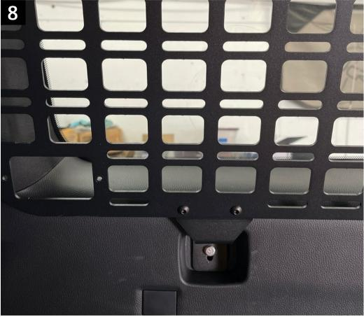
With your brackets loosely bolted into place, bolt your molle panel to the lower bracket using the provided 1/4" button heads and a flange nuts.
