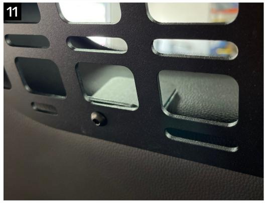
Take the provided double sided 3M tape and cut to size of the last remaining brackets. Once cut to size peel one side of the tape off and place on the bottom side of the bracket, as shown above. Peel the other side of the tape, and feed the bracket through the logo hole and shimmy down to the mounting hole on the bracket and stick to the plastic and bolt into place.
