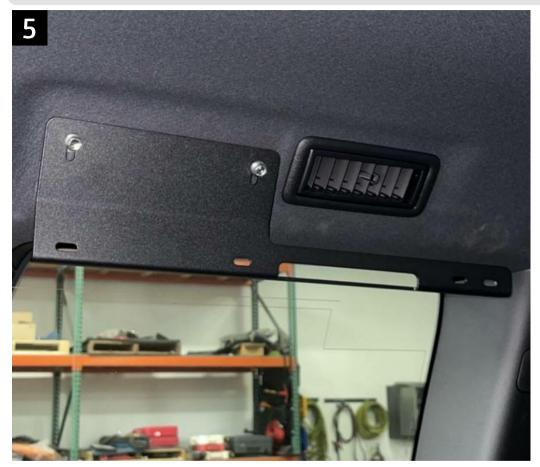
Now take the provided upper bracket and bolt them into the factory holes that held the handle into place, using the factory hardware. The handles can be installed over the shown. Longer M6 hardware is provided if extra thread engagement is needed for your brackets or left off. Install as shown in the orientation above. Leave this loose for now for adjustment.
