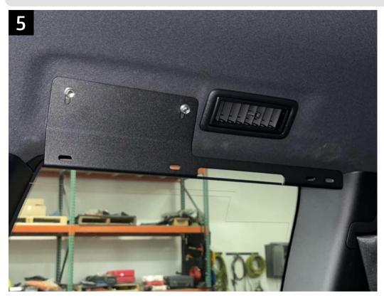
Now take the provided upper bracket and bolt them into the factory holes that held the handle into place, using the factory hardware. The handles can be installed over the shown. Longer M6 hardware is provided if extra thread engagement is needed for your brackets or left off. Install as shown in the orientation above. Leave this loose for now for adjustment.
