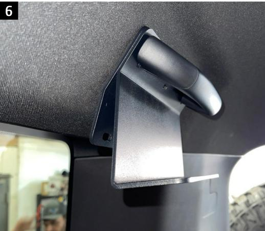
If installing an upper shelf, stack the mounting bracket over the molle panel bracket as setup.
