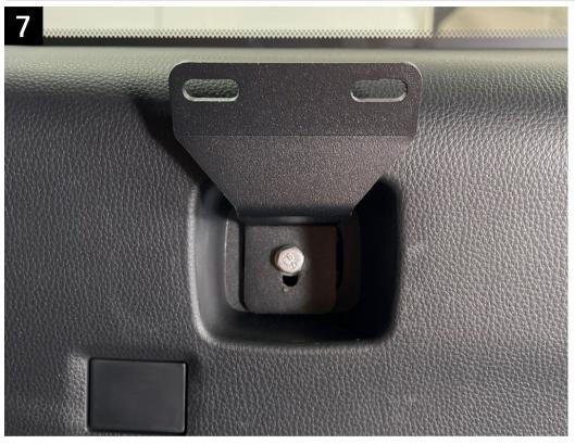
Take the provided lower bracket and bolt it into place in the orientation shown above, using the provided long m6 bolt and spacer behind the bracket. Leave this loose for now so you can have adjustment if needed.
