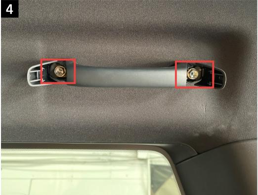
Next, you need to remove the grab handles from each side of the vehicle. Pop off the plastic covers and remove the (2) factory hex bolts using a 10mm socket. Repeat this on each side of the vehicle.
