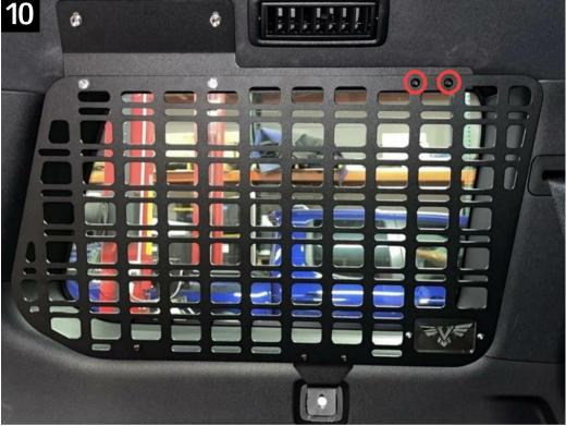
Next, take the provided 1/4" hex heads with a washer and flange nut and bolt them to the top back bracket as shown above using a 7/16" wrench.
