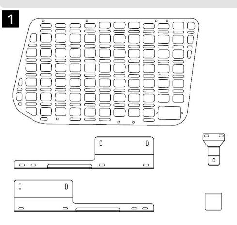
Included Hardware: 3x M6 x 40mm Hex Head Bolt | 5x 1/4" Washer | 3x 1/4"-20 x 1/2" Button Head Bolt | 9x 1/4"-20 Serr. Flange Nuts | 2x 1/4"-20 x 3/4" Button Head Bolt | 2x 1/4"-20 x 1" Hex Head Bolt | 1x 1/2" OD Spacer | 2x VHB Adhesive
