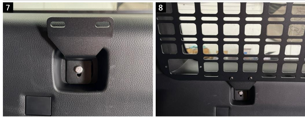
Take the provided lower bracket and bolt it into place in the orientation shown above, using the provided long m6 bolt and spacer behind the bracket. Leave this loose for now so you can have adjustment if needed.
