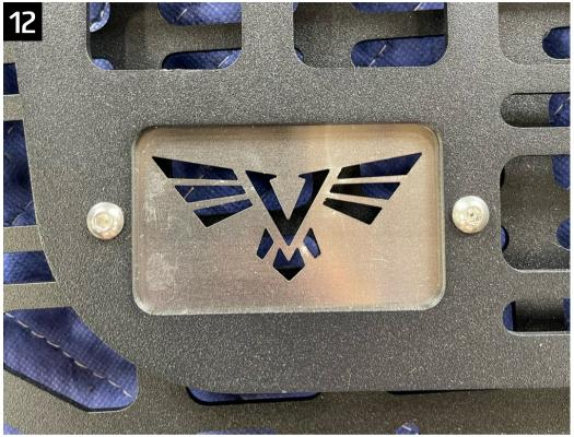
To complete the install, take the provided stainless steel logo plate and bolt it into the cut out in the molle panel with the provided smaller button heads. Shown in the orientation above. Be sure to tighten any loose hardware.
