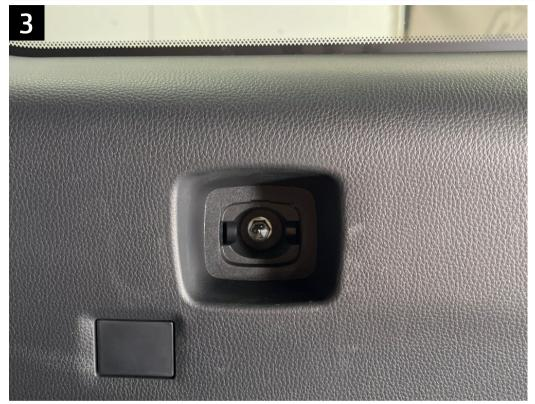
Start by removing the plastic cover, below the rear window, with a pry tool or a flat head screw driver. Once removed, use a 10mm socket to remove the hex bolt. Be sure to hold onto this for later use.
