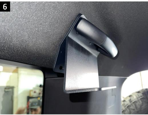
If installing an upper shelf, stack the mounting bracket over the molle panel bracket as setup.
