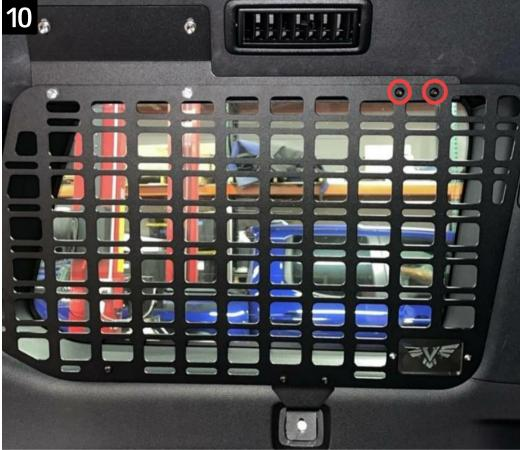
Next, take the provided 1/4" hex heads with a washer and flange nut and bolt them to the top back bracket as shown above using a 7/16" wrench.
