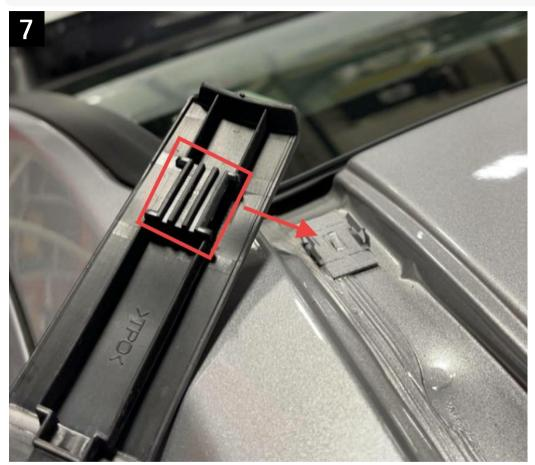
This image shows the clipping mechanism of the rubber trim.
