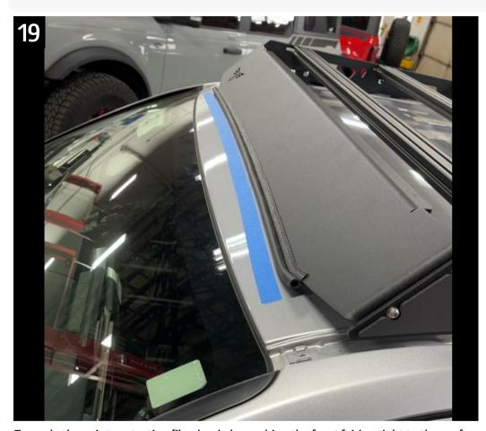
To apply the paint protection film, begin by pushing the front fairing tight to the roof and apply tape 1/8" - 1/4" from the edge, anywhere it contacts the roof.
