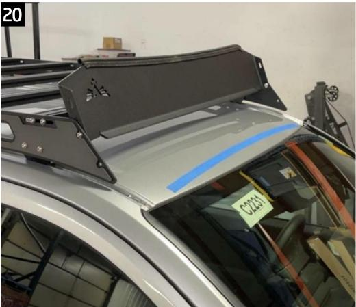
Remove the bottom bolt and flip the fairing up and out of the way. Then, apply paint protection film edge to edge with the tape line previously laid out.
