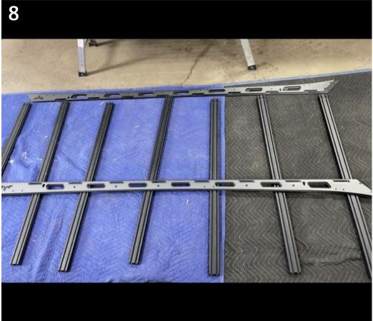
To begin the rack assembly, first mount the accent plate to the side rails using the black 1/4"-20 bolts, nuts and black 1/4" washers. This hardware should be used in each of the 5 single holes located under the center of the cross bar slots on each side rail.
