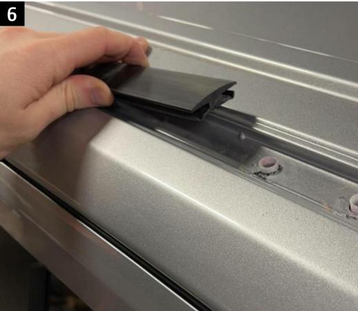
Pull the forwardmost piece of rubber trim out of the gutter. The front end is clipped into a small metal bracket. Pry up to remove the trim from the clip.
