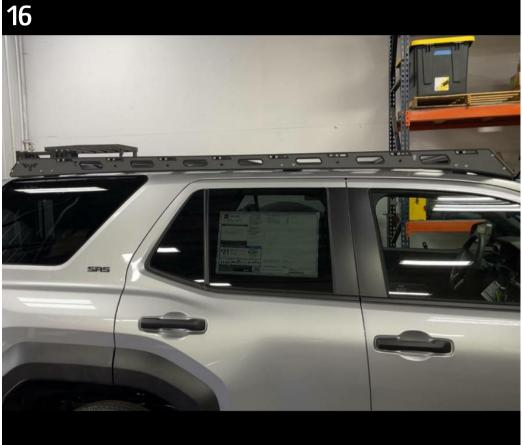
Set the rack up into place and loosely mount attach it to each of the mounts using the 1/4" hardware. Once this is achieved, the mid and rear mounts can be tightened fully to the roof. Be sure to do this before the RTV hardens.
