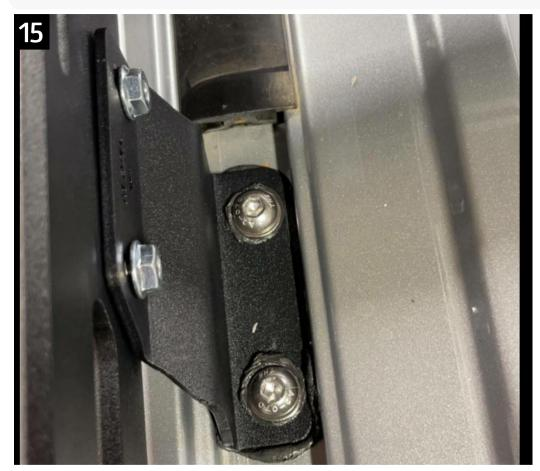
Next, mount the mid and rear mounts to the vehicle. Begin by putting a bead of RTV around the mounting holes in the roof and then set the mount into place. Put a bit more RTV over the holes themselves so that the bolts have to pass through it. Then, loosely install the M8 bolts and washers into the roof of the vehicle.
