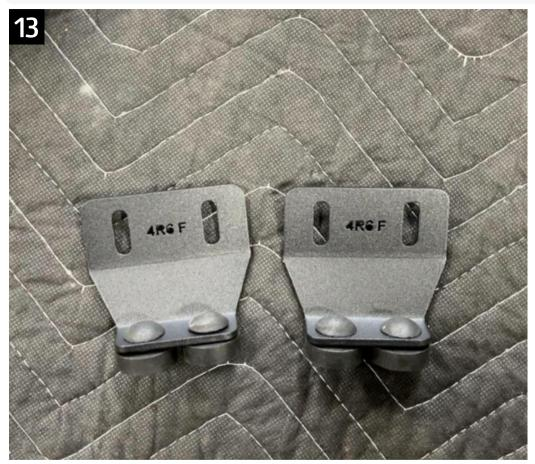
Pop the rubber bumpers into the bottom of the front mount. It is easiest to get part of the edge in through the hole and then push and twist to fully seat it.
