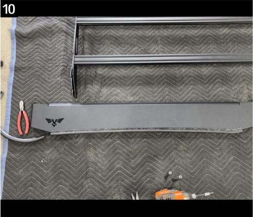
Mount the strip of trim to the bottom edge of the front fairing. Start just to the outside of the peak of the bottom edge and continue until it reaches the equivalent point on the other side of the fairing. Cut off any extra.
