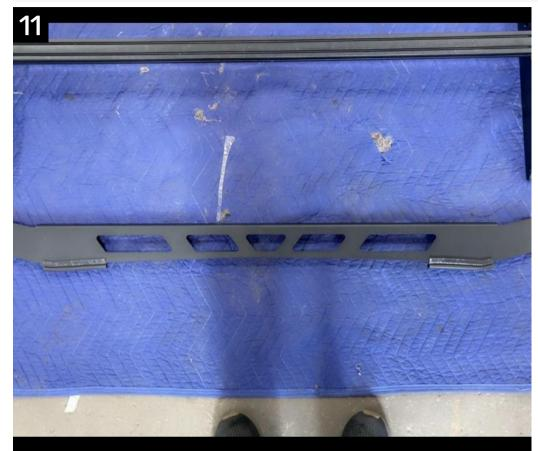
Cut the extra trim as needed and mount it onto the bottom edge of the rear fairing wherever it contacts the roof of the vehicle. It may be necessary to cut it into 2 pieces put one on each peak of the fairing.
