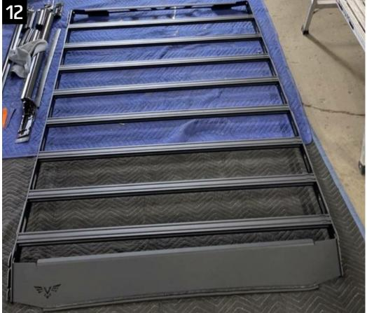
Next, mount the front and rear fairings. To do this, use the 1/4"-20 X 3/4" button head bolts, 1/4" washers, and 1/4"-20 serrated flange nuts. The front fairing will need 3 of each per side and the rear fairing will need 2 of each per side. When mounting the front fairing, adjust it all the way up to avoid contact with the roof and tighten for now. Repeat this step for the rear fairing.
