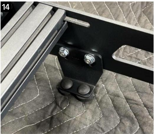
Install the front mounts onto the rack using the 1/4" hardware. Push it all the way down and tighten it for now.
