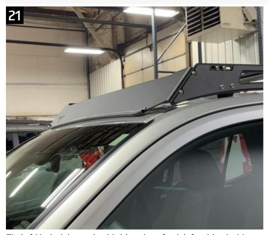
Flip the fairing back down and push it tight to the roof again before tightening it into place. Repeat these steps for the rear fairing as well.
