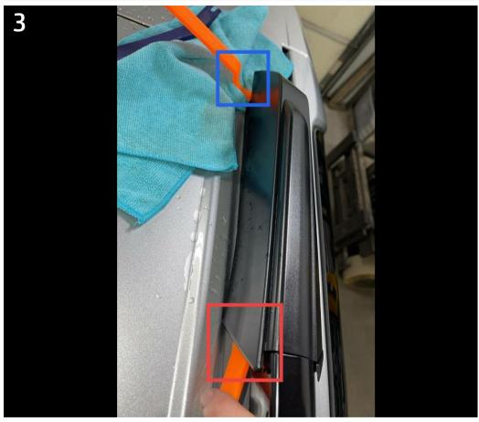
Start by inserting a tool into the area boxed in red in the image. Pry towards the center of the vehicle until there is a pop of the clip coming undone. Leave a tool there to prevent the clip from reattaching and insert another tool under the bottom edge boxed in blue. Again, pry until the clip comes undone.
