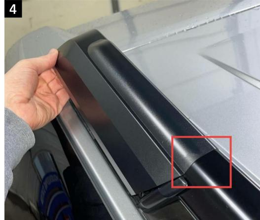
The cap can then be gently pulled away from the center of the vehicle to undo the two clips on the other side. There are also plastic fingers sticking into the area boxed in red, so the cap will need to be pulled out from there.
